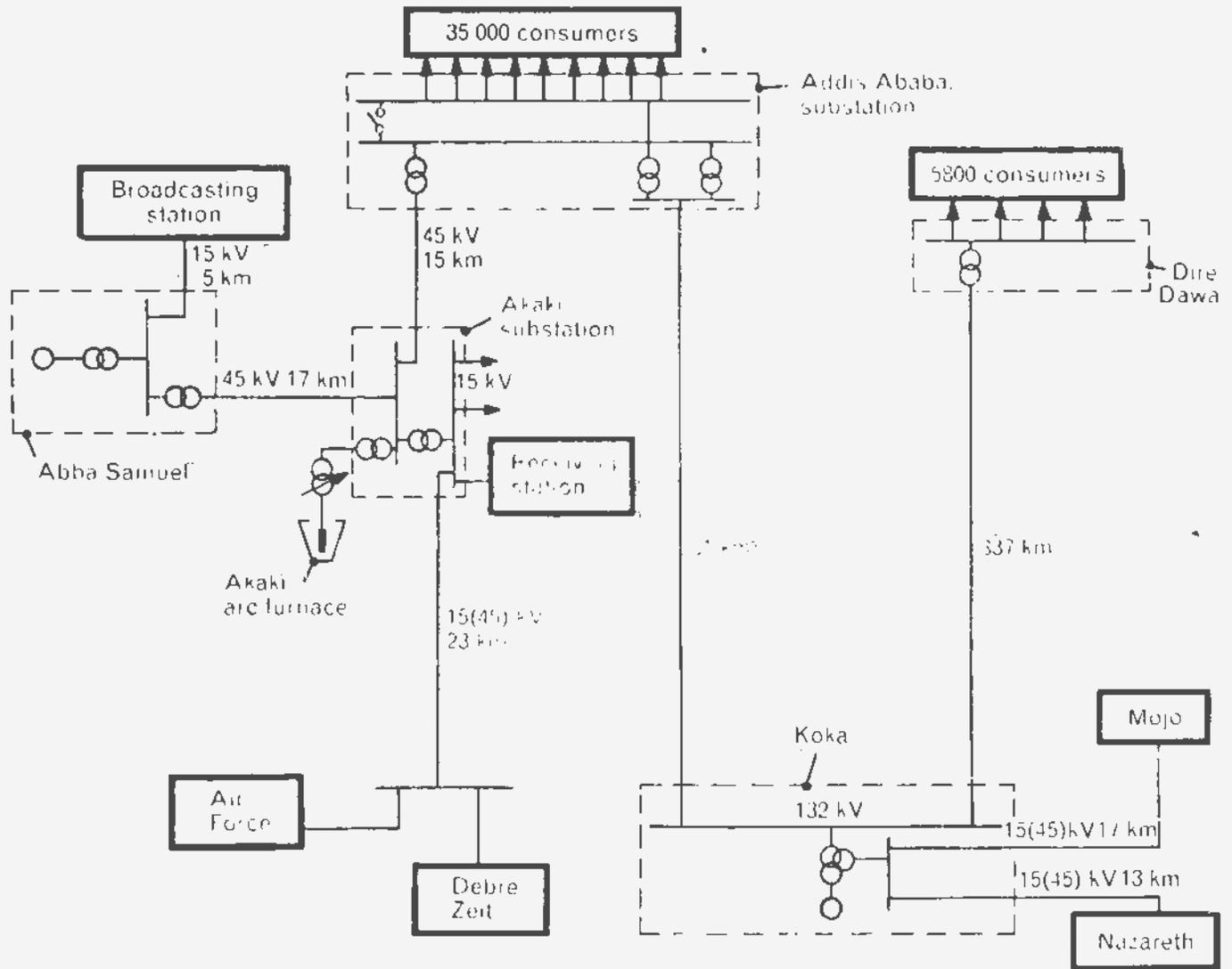
Fig. 1. — Simplified Single Line diagram of the power system around Addis Ababa.
