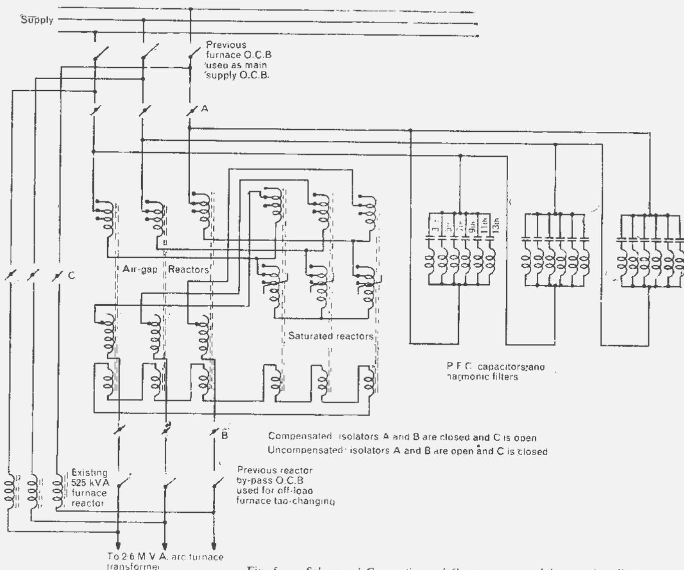
Fig. 5. - Scheme of Connections of Compensator and furnace installation
