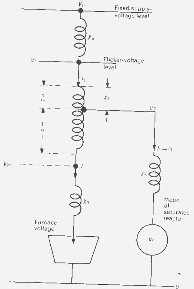
Fig. 4. — Equivalent circuit of compensator.
