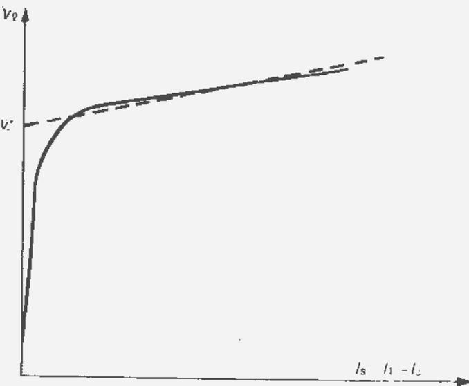
Fig. 3. — Voltage/Current Characteristic of saturated reactor.
