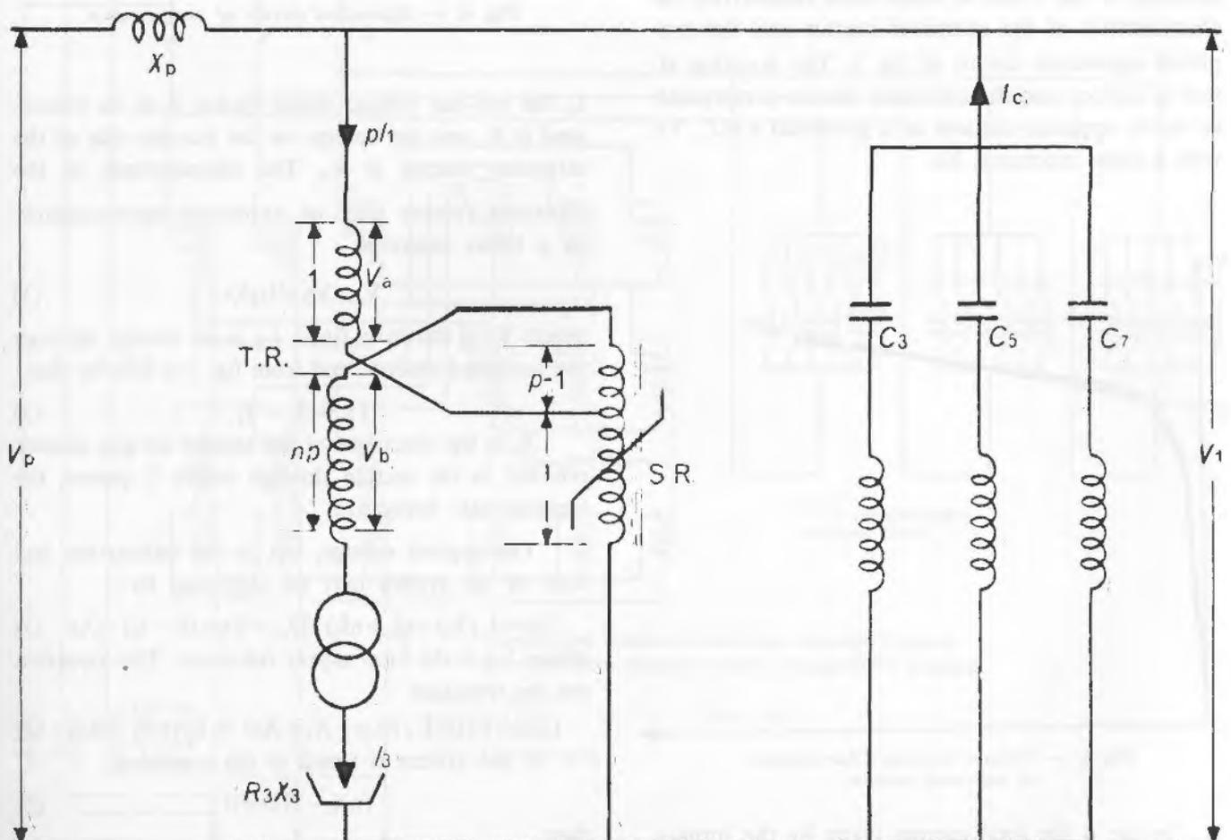
Fig. 2. — Single-phase diagram of flicker compensator including internal voltage boosting.
