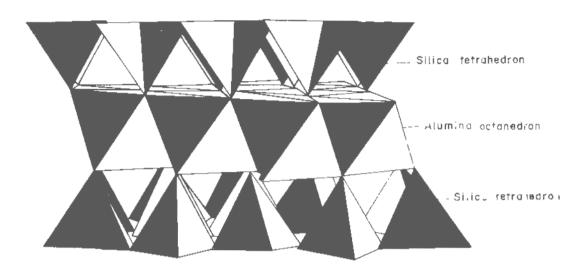
Fig. 1 Model of a Layer of Montmorillonite after Philip Low [4]
