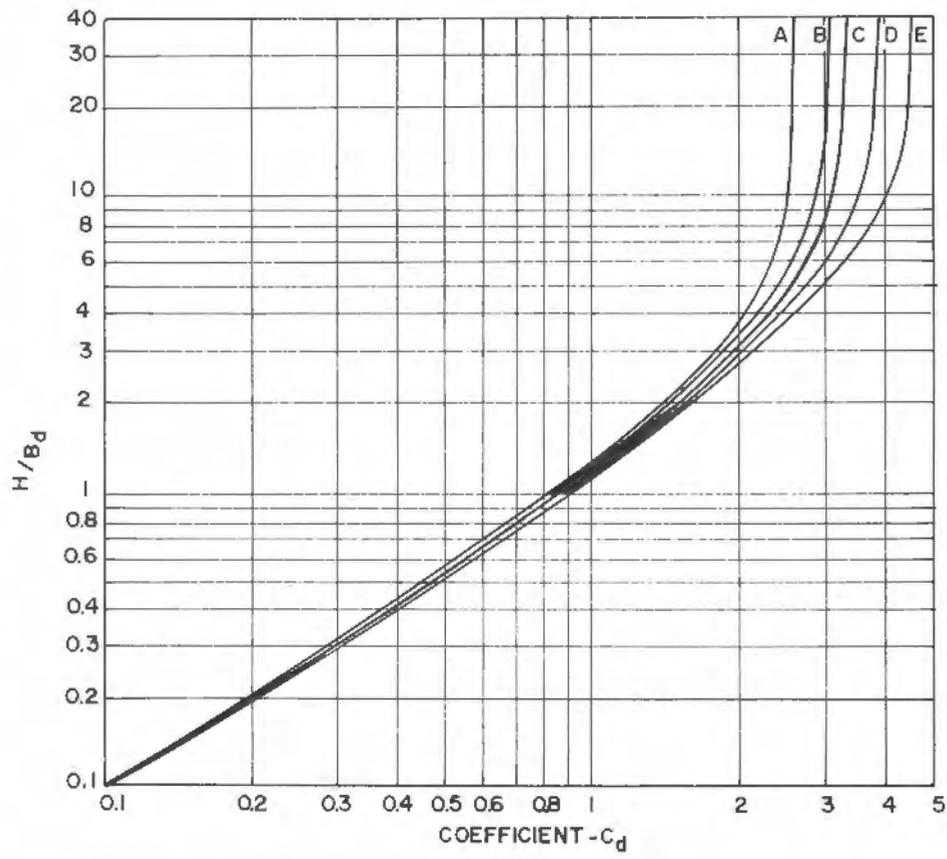
Fig. 5. Graph for determining  $C_d$  coefficients
