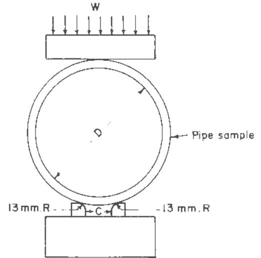
Fig. 3. Crushing Test Assembly (3-edge bearing)
