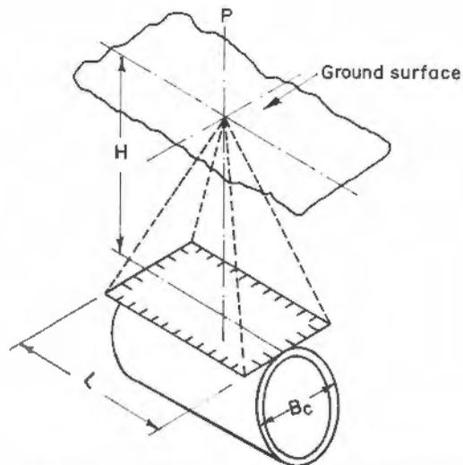
Fig. 6. Concentrated superimposed load
