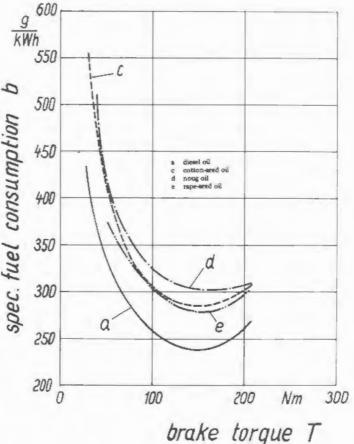
Fig. 3 Specific fuel consumption as functions of the brake torque at 1600 rpm. Comparison between esterified vegetable oils and diesel oil Vegetable Oils for Diesel Oil
