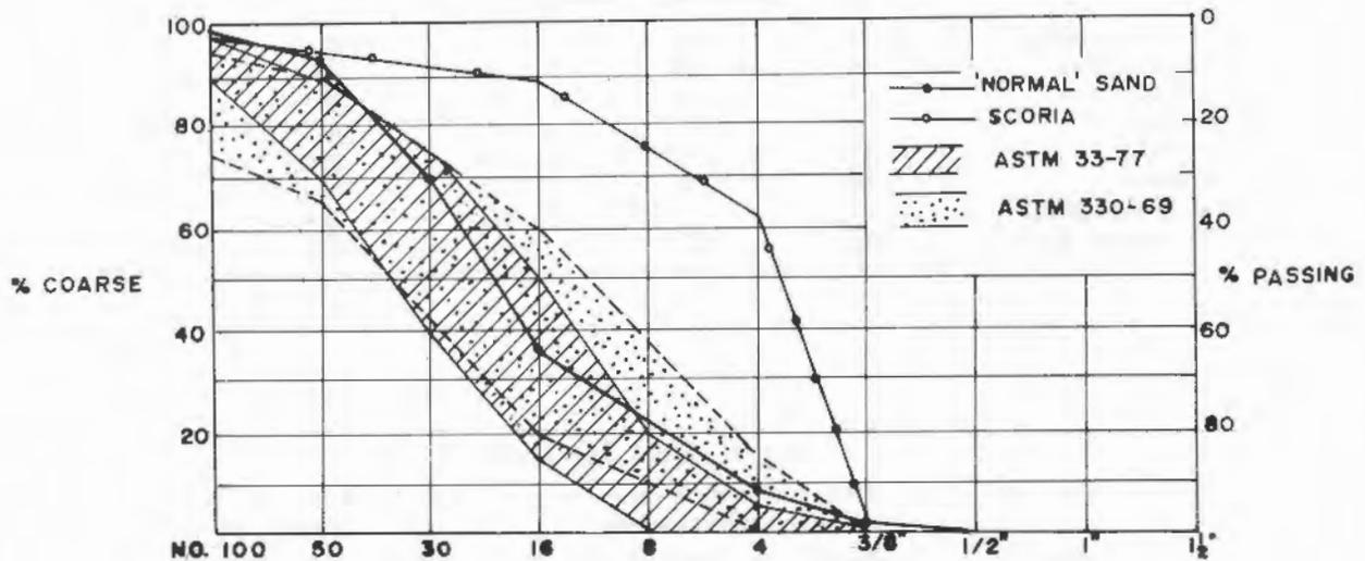
Fig. 3 Grain Distribution of Normal and Scoria Sand
