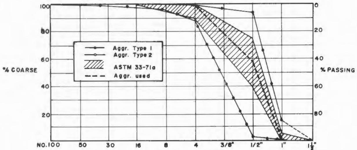
Fig. 2 Grain Distribution of Blended Coarse Aggregates
