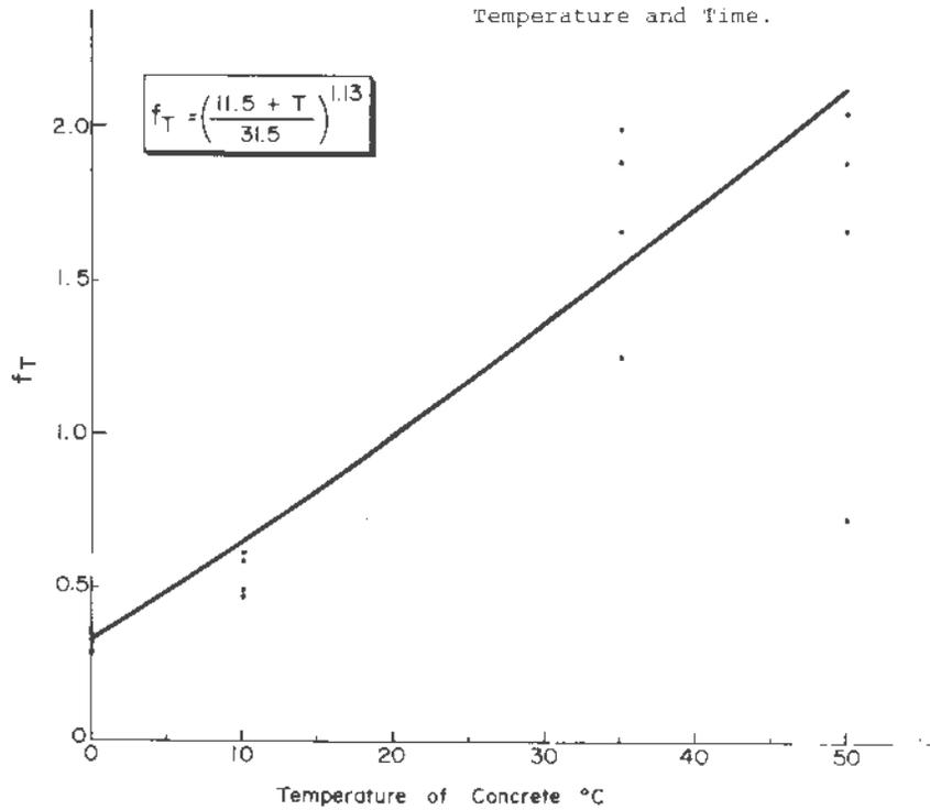
Fig. 2. Maturity Function for Calculating Equivalent Curing Age at 20°C.
