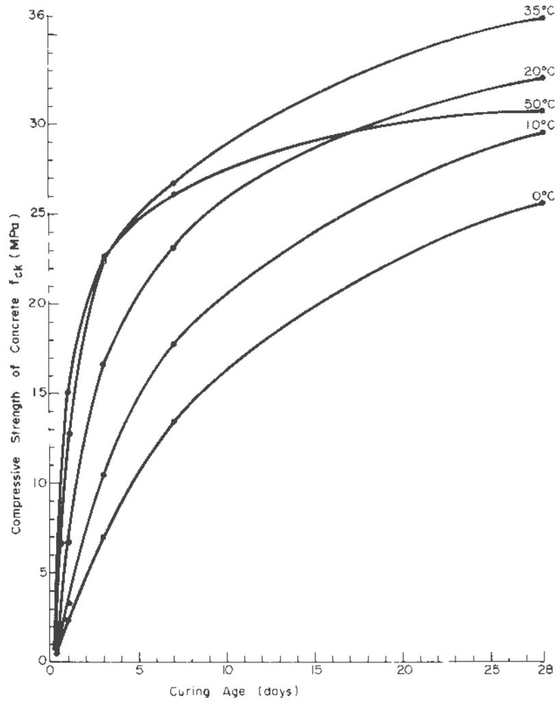
Fig. 1. Strength Development of Concrete in Relation to Temperature and Time.
