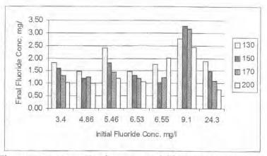
Figure 1 Dependence of optimum dose on initial fluoride concentration
