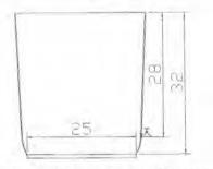
Figure 4 Final design for fluoride concentration of less than 10%, all <u>units in cm</u>.
