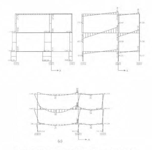
Figure 7 Internal forces and moments in the fixed-base model: (a) axial force; (b) shear force; (c) bending moment
