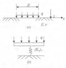
Figure 2 (a) An ideally flexible rectangular footing on the surface of an elastic half space;
