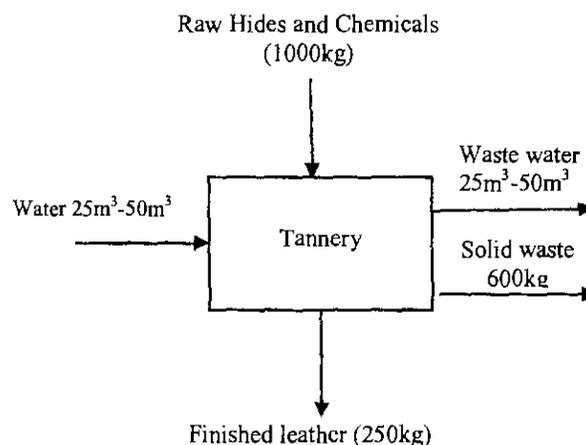
Figure 1 Schematic diagram for inputs and outputs of a typical leather industry
