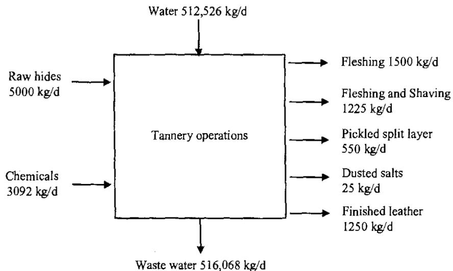
Figure 3 Inputs and outputs of tanning operation in Addis Ababa Tannery
