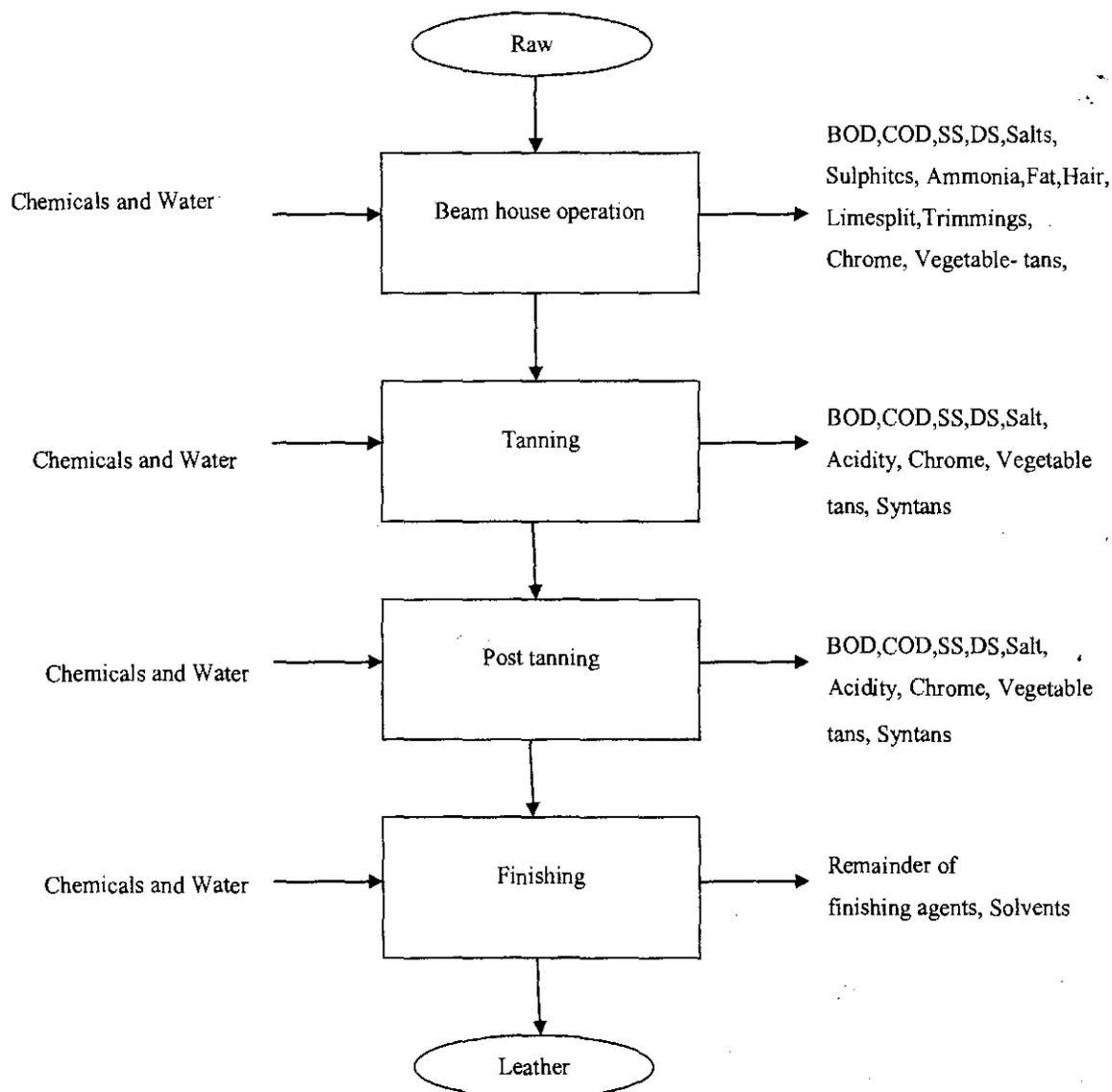
Figure 2 Process flow diagram for the main tannery operations
