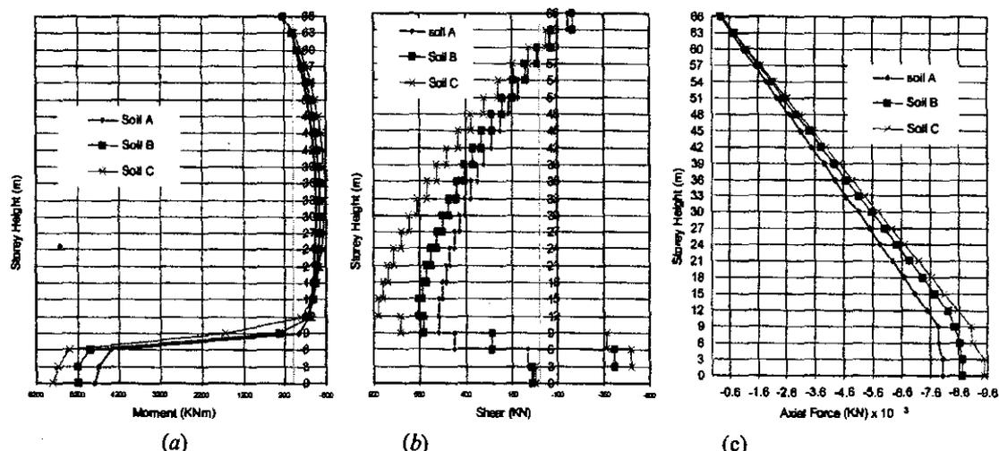
Figure 10 Height-wise variation of internal forces in Shear Wall SW2 for fixed- and flexible-base models of Structural System 3 for an embedment depth of 3 m in the different soil types: (a) moment; (b) shear; (c) axial force
