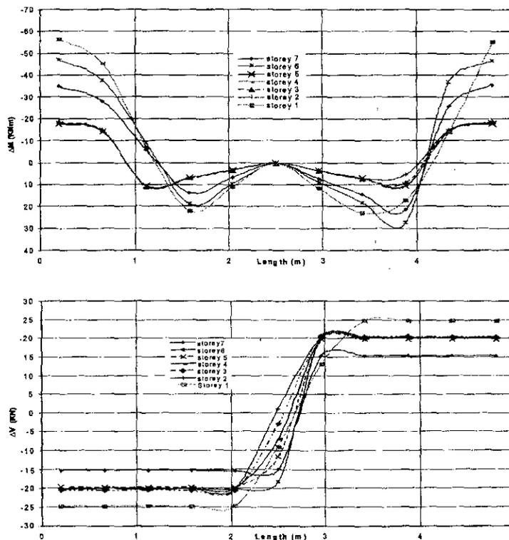
Figure 3 Plots showing difference in bending moment (upper) and in shear force (lower) along the length of end-bay beams in all floors of Structural System 1 for embedment depth of 1 m in Soil Type C.
