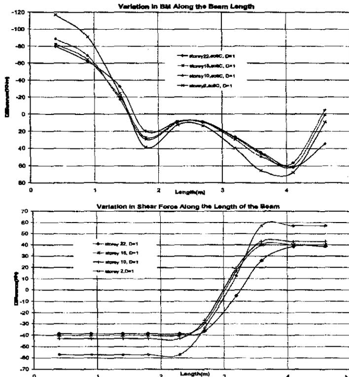
Figure 8 Plots showing differences in bending moment, and shear force along the length of selected end-bay beams of Structural system 3 for embedment depth of 1 m in Soil Type C
