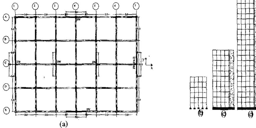
Figure 2 (a) Floor plan of all buildings studied; (b) Structural System 1 (6-stories); (c) Structural System 2 (11-stories); (d) Structural System 3 (21-stories)
