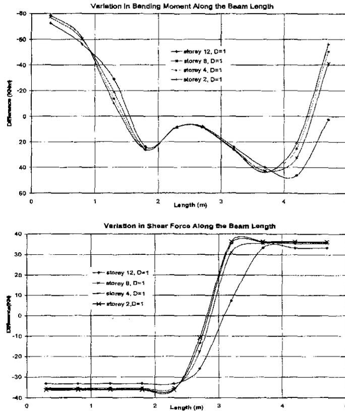
Figure 4 Plots showing differences in bending moment and shear force along the length of selected end-bay beams of Structural system 2 for a foundation embedment depth of 1 m in Soil Type C
