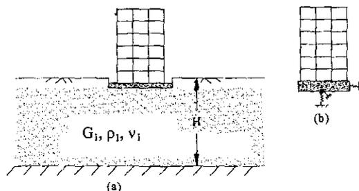
Figure 1 a) The building embedded in a layered formation; b) The building model with base springs
