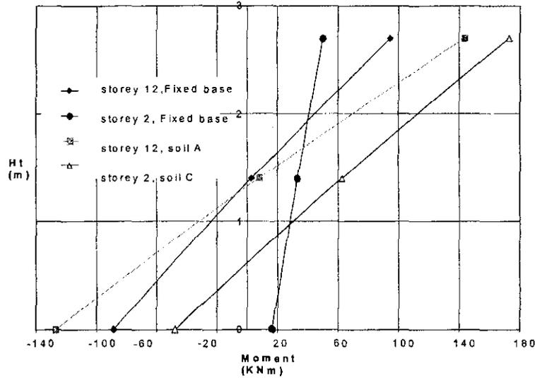
Figure 6 Bending moment variations in a column for selected cases of the fixed- and flexible-base models
