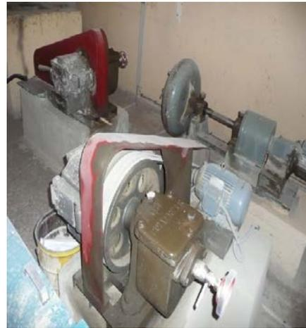
Figure 1 Grinding mill used for grinding and preparing cement (Photo from Mughar Cement Factory Laboratory).
