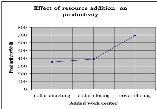
Figure 5 Effect of three extra effective work centers on productivity
