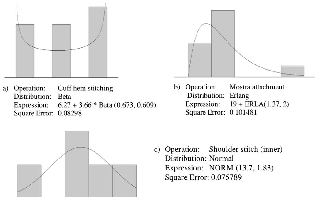
Figure 2 Examples of distribution type of operations (using Arena input Analyzer)
