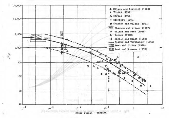
Fig. 8 In-situ shear moduli for saturated clays [5]
