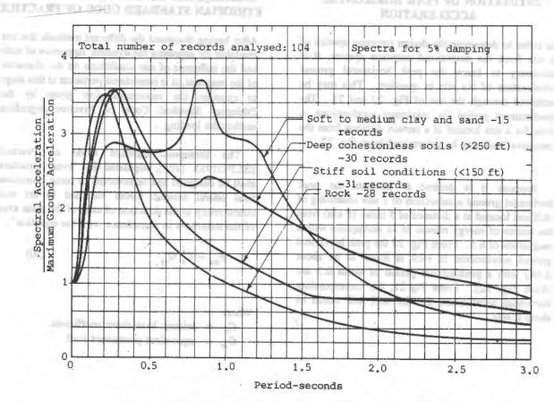
Fig. 17 Percentile acceleration spectra for different aite conditions [9]
