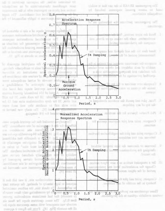
Fig. 15 Determination of normalized acceleration response spectrum [1]
