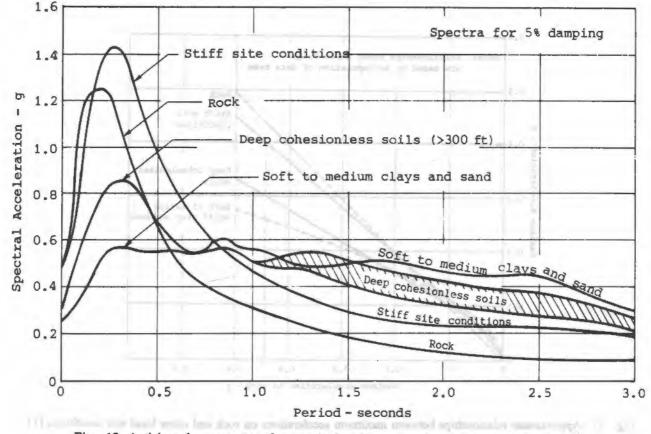
Fig. 19 Anticipated mean spectra for magnitude 6 1/2 earthquake at distance of 5 miles [9]
