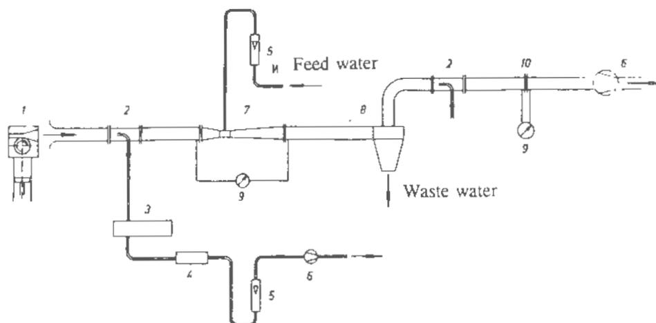
Figure 1 Structure of the Experimental Unit; 1-Dust dosing system, 2-Sampling, 3-Scattered light measuring unit, 4-Filter, 5-Rotameter, 6-Blower, 7-Venturi scrubber, 8-Drop separator, 9-Manometer, 10-Measuring shade
