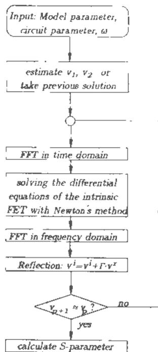
Figure 4 Flow Diagram of the Simulation
