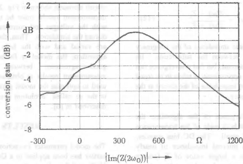
Figure 5 Calculated Maximum Achievable Conversion Gain of a 16 to 32 GHz Frequency Doubler Circuit as a Function of Second Harmonic Load Reactance.
