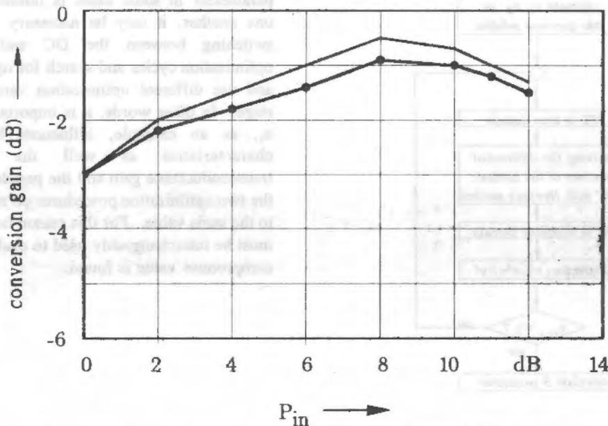
Figure 6 Measured and Simulated Conversion Gain of a 16 to 32 GHz Frequency Doubler Circuit as a Function of the Input Fundamental Power
