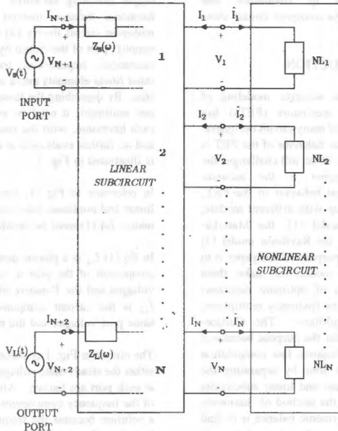
Figure 1 A Nonlinear Microwave Circuit, Divided into Linear and Nonlinear Subcircuits, with the Source and Load Impedances Absorbed into the Linear Subcircuit.
