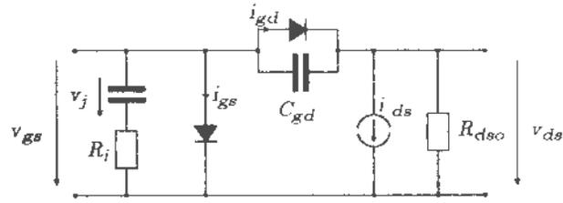
Figure 2 The Nonlinear Transistor Model
