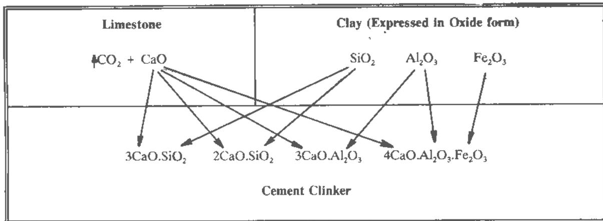
Figure 6 Transformation of Cement raw Material to clinker
