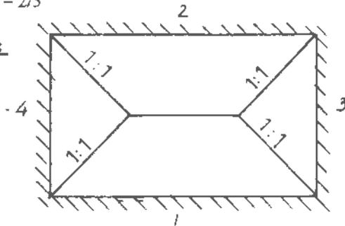
Figure 11 Slab panel continuous along all four sides
