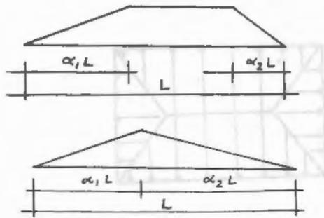
Figure 2 Trapezoidal and triangular loadings
