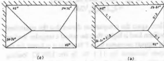
Figure 16 Load dispersion (a) as obtained by the yield line analysis for isotropic slab, (b) as recommended by the ESCP2.
