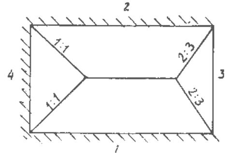
Figure 9 Slab panel simply supported along one of the shorter sides only.
