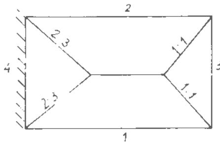
Figure 5 Slab panel continuous along one of the shorter sides only
