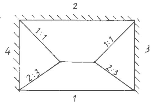
Figure 10 Slab panel simply supported along one of the longer sides only
