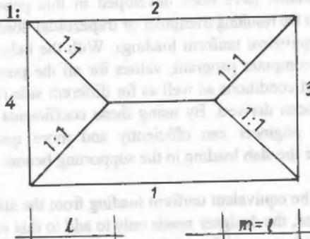
Figure 3 Slab panel simply supported on all four sides
