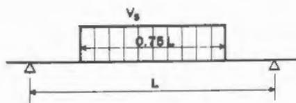
Figure 14 Distribution of Load on a Beam Supporting a Two-Way Spanning Slab
