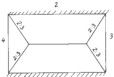
Figure 8 Slab panel continuous along the two shorter sides only
