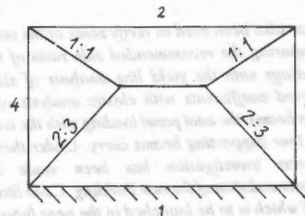
Figure 4 Slab panel continuous along one of the longer sides only.
