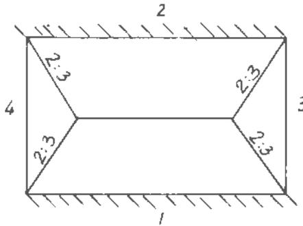
Figure 7 Slab panel continuous along the two longer sides only.
