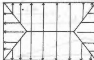
Figure 1 Load dispersion from slab to the four supporting beams
