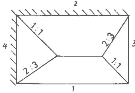
Figure 6 Slab panel continuous along the two adjacent sides only
