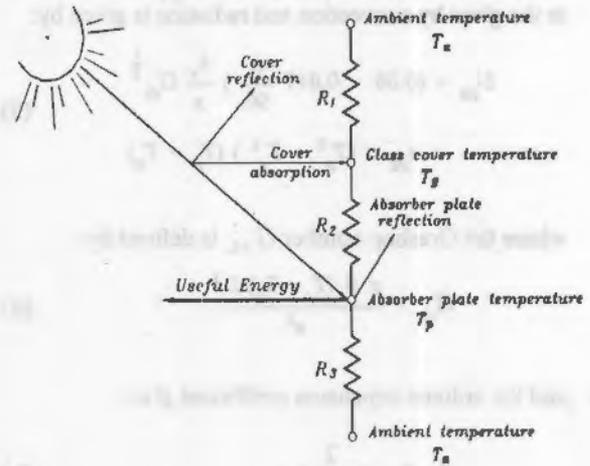
Figure 2 Thermal circuit for solar collector
