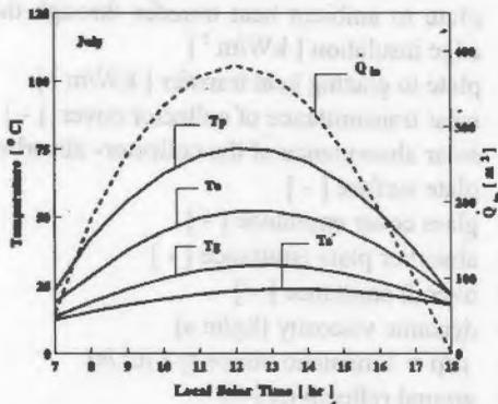
Figure 6 Ambient, glass, collector outlet & plate temperatures for July
