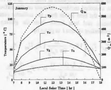
Figure 4 Ambient, glass, collector outlet and plate temperatures for January
