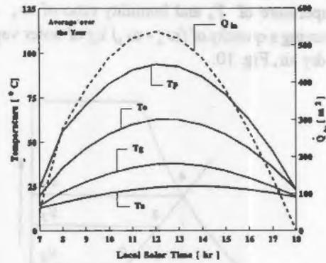
Figure 8 Average yearly values of temperatures and solar flux
