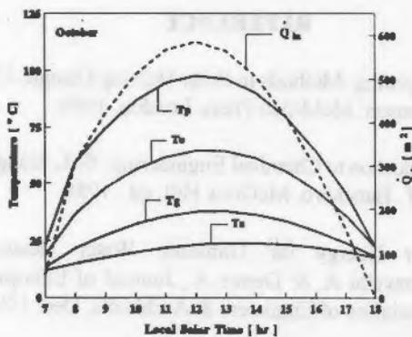
Figure 7 Ambient, glass, collector outlet & plate temperature for October
