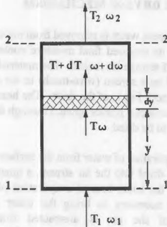
Figure 3 Heat and material balance in a dryer
