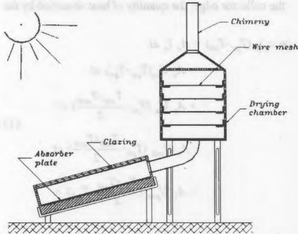
Figure 1 Integrated solar collector and drying chamber
