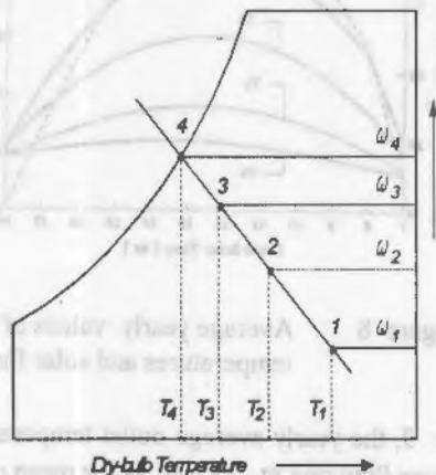
Figure 10 Psychrometric representation of drying mechanism
