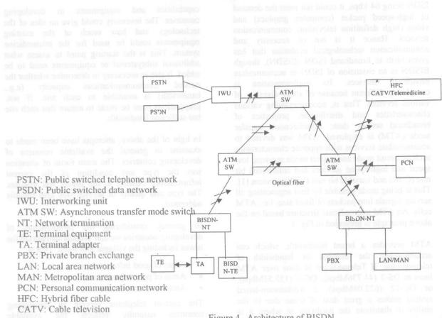
It was designed to make Broadband-ISDN (B-ISDN) a reality. B-ISDN was created conceptually as just an extension of ISDN so it functions as a communication network that can provide integrated broadband services such as high-speed-data service, video phone, video conferencing, CATV services along with traditional ISDN services such as phone and telex.
