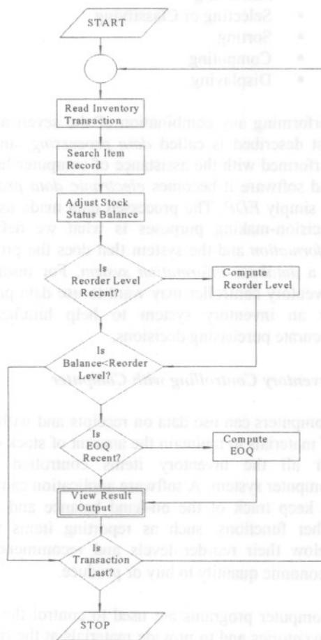
Fig. 7 Flowchart of a Computerized Inventory System
