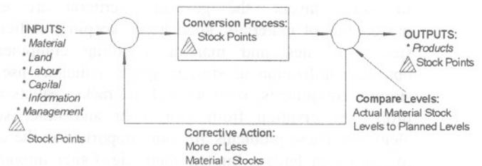
Fig. 1 Material Conversion Process
