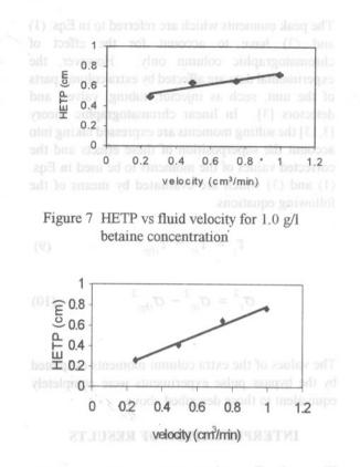
Figure 8 HETP vs fluid velocity for 2.0 g/l betaine concentration
