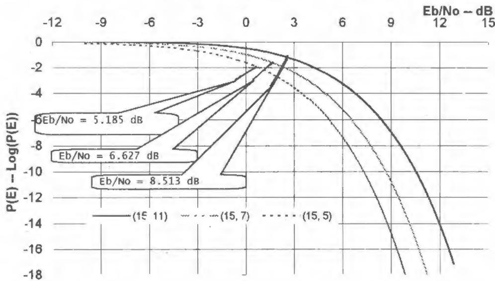
Figure 5 Plot of error Probability of the Codes
