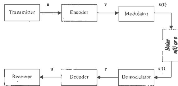
Figure 1 Error Control Coding path
