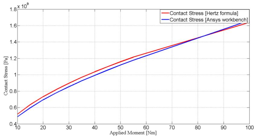
Fig. 5: Contact Stress Distribution of FEM and Hertz Equation with Error
