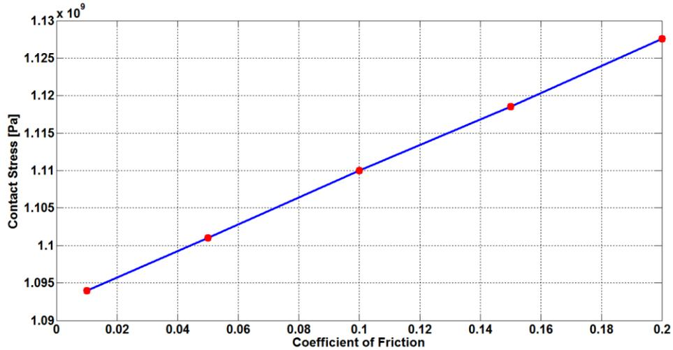
Fig. 4: Influence of Coefficient of Friction on Contact Stress
