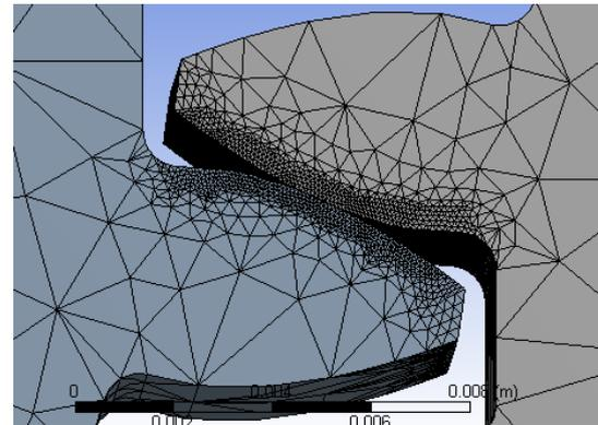
Fig. 2: Fine Mesh Near the Contact of FEM Analysis
