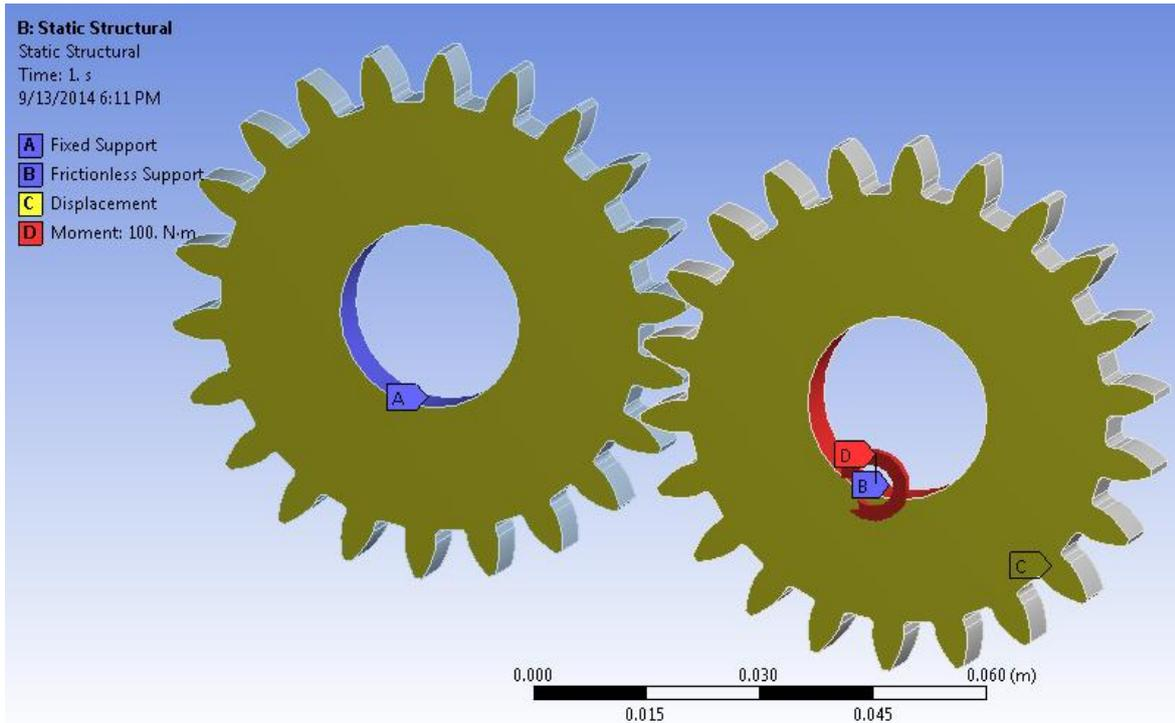
Fig. 1: Assembly of Meshing Pinion and Gear
