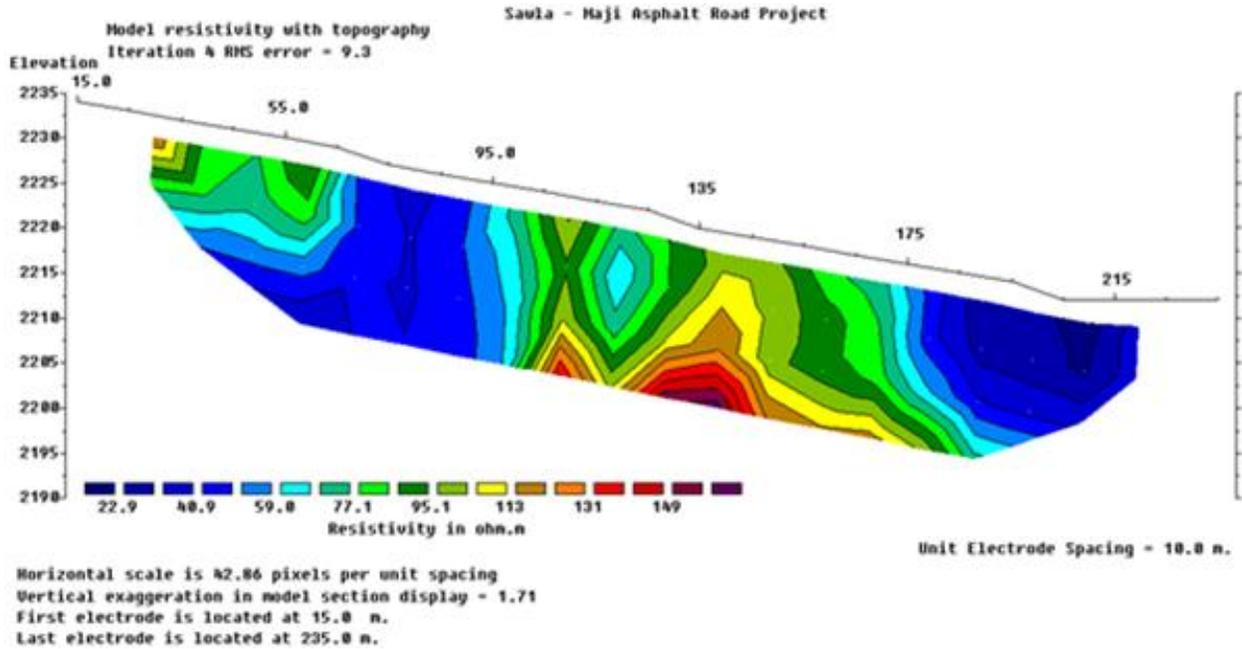
Fig. 2: Resistivity Result at Station 24+500 – 24+720
