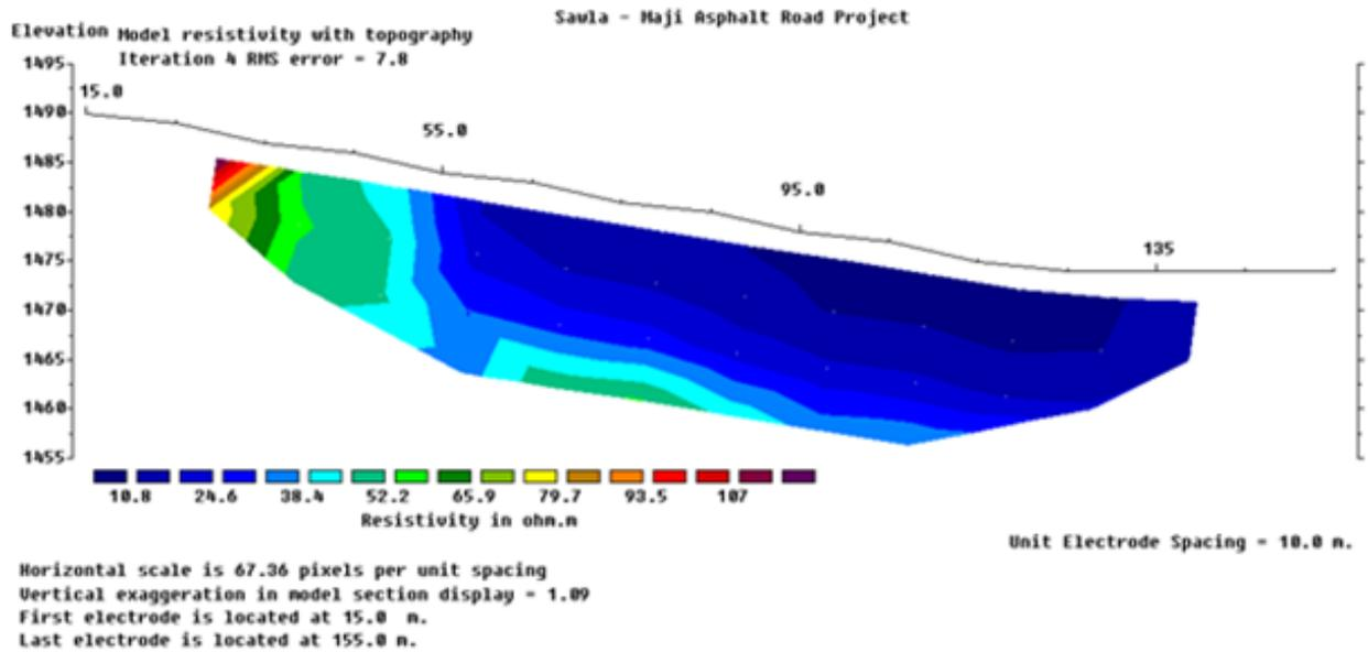
Fig. 3: Resistivity Result at Station 33+000 – 33+140
