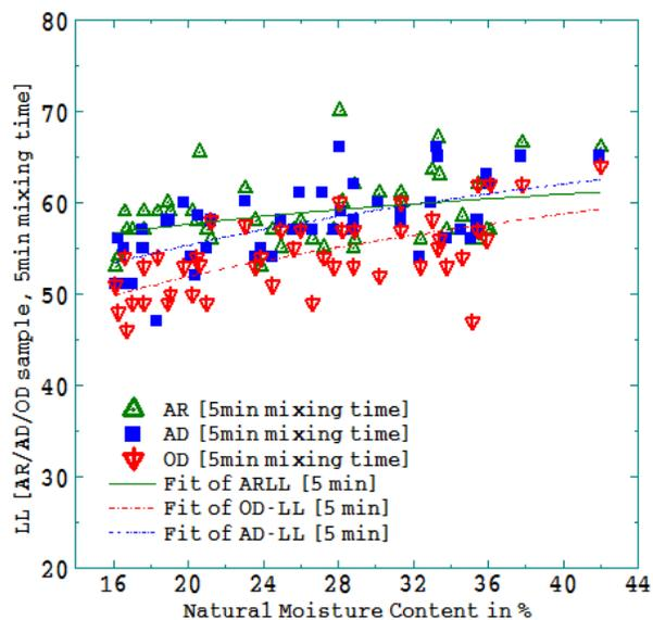
Fig. 11. Variations in liquid limits on AR,AD and OD Group A Ethiopian laterite soils tested at 5min mixing time
