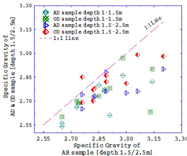
Fig. 14. Line of equality between specific gravity values for different pretest drying treatments
