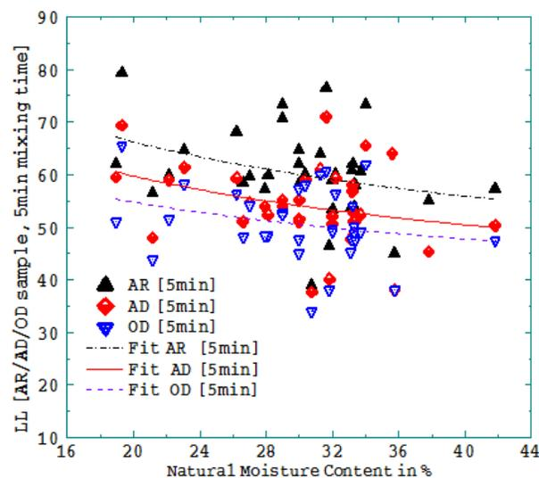
Fig.12. Variations in liquid limits on AR, AD and OD Group B Ethiopian laterite soils tested at 5min mixing time
