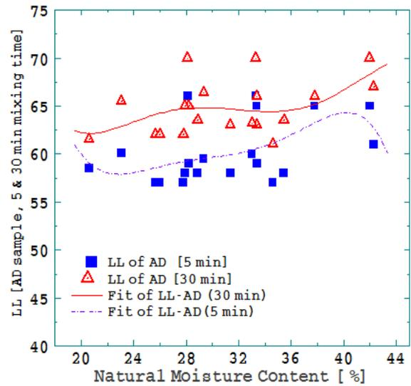
Fig. 8. Variations of liquid limit using AD soil sample tested at 5 and 30min mixing time with natural moisture content for TWR laterite soils tested.
