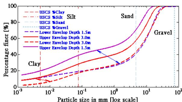
Fig.17. Grading envelop for silty gravel with sand textured laterites with depth for various AR pretreatment conditions
