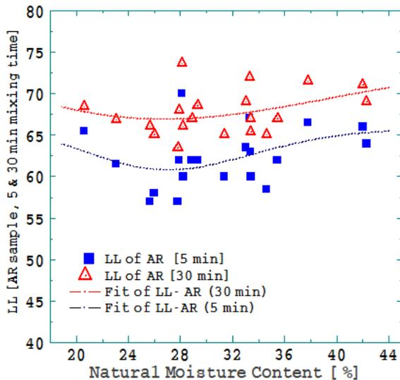
Fig. 7. Variations of liquid limit using AR soil sample tested at 5 and 30min mixing time with natural moisture content for a range of TWR laterite soils tested
