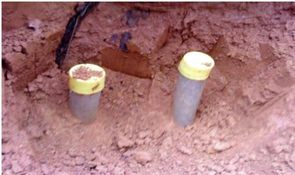
Fig. 3 Typical undisturbed sampling using a thin wall tube sampler around *Nejo* in western Ethiopia
