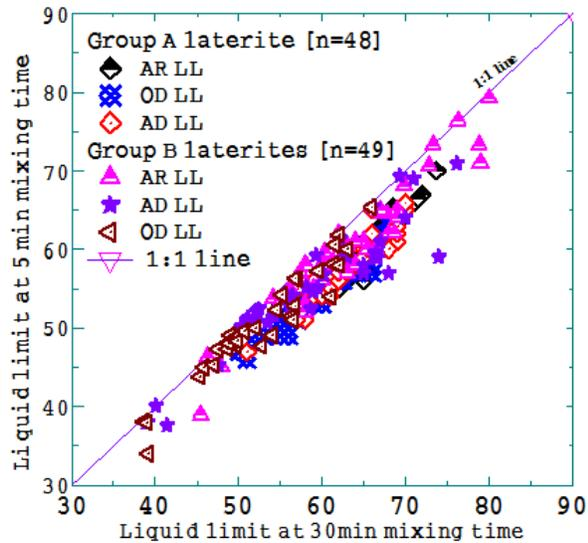
Fig. 13. Liquid limit between 5 and 30min mixing time on AR, AD and OD samples for Group A and Group B TWR laterite soils of Ethiopia
