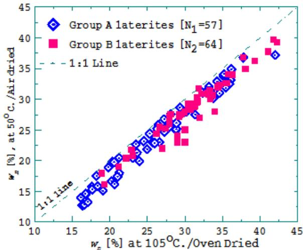
Fig. 6. The relationship between natural moisture content using oven drying of 50°C and 105°C for a range of TWR laterite soils of Ethiopia.
