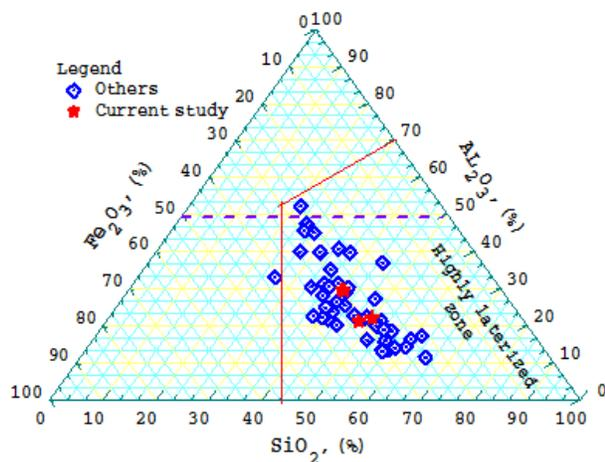
Fig. 5.  $SiO_2 - Al_2O_3 - Fe_2O_3$  triangular diagram indicating the position of the degree of laterization of Ethiopian laterites.
