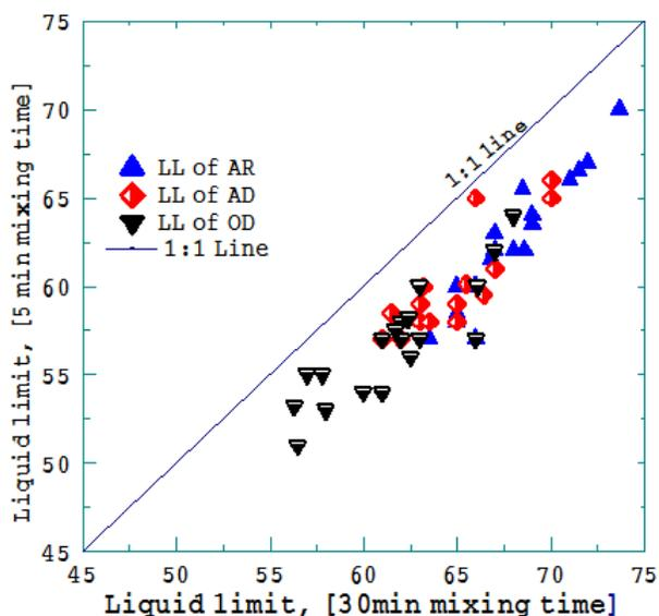
Fig. 10. The relationship between liquid limits using 5 and 30 min mixing time on AR, AD and OD for laterite soils tested
