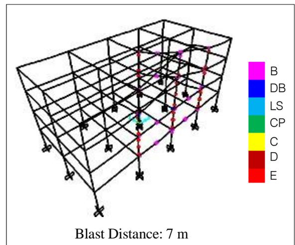
Fig. 5: Hinges and Deformed Shape for Various Standoff Distances
