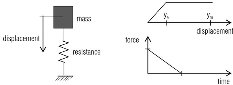
Fig. 2 Simplified elasto-plastic SDOF model for blast load analysis [4]
