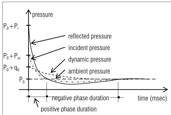
Fig. 1 Complete Over-Pressure – Time Profile [6]
