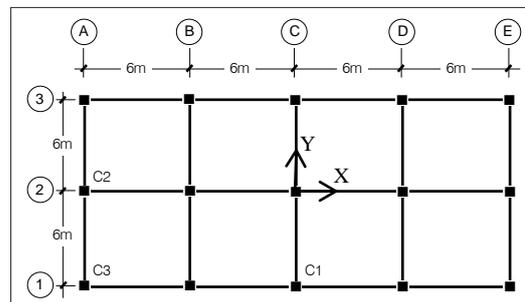
Fig. 3: RC Building Plan and Location of Removed Columns.
