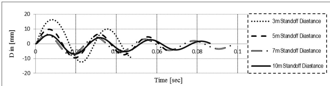
Fig. 7: SDOF Blast Analysis Deformation Response at Different Standoff Distances
