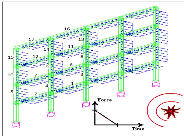
Fig. 4: Distribution of Blast Load on Structural Elements.
