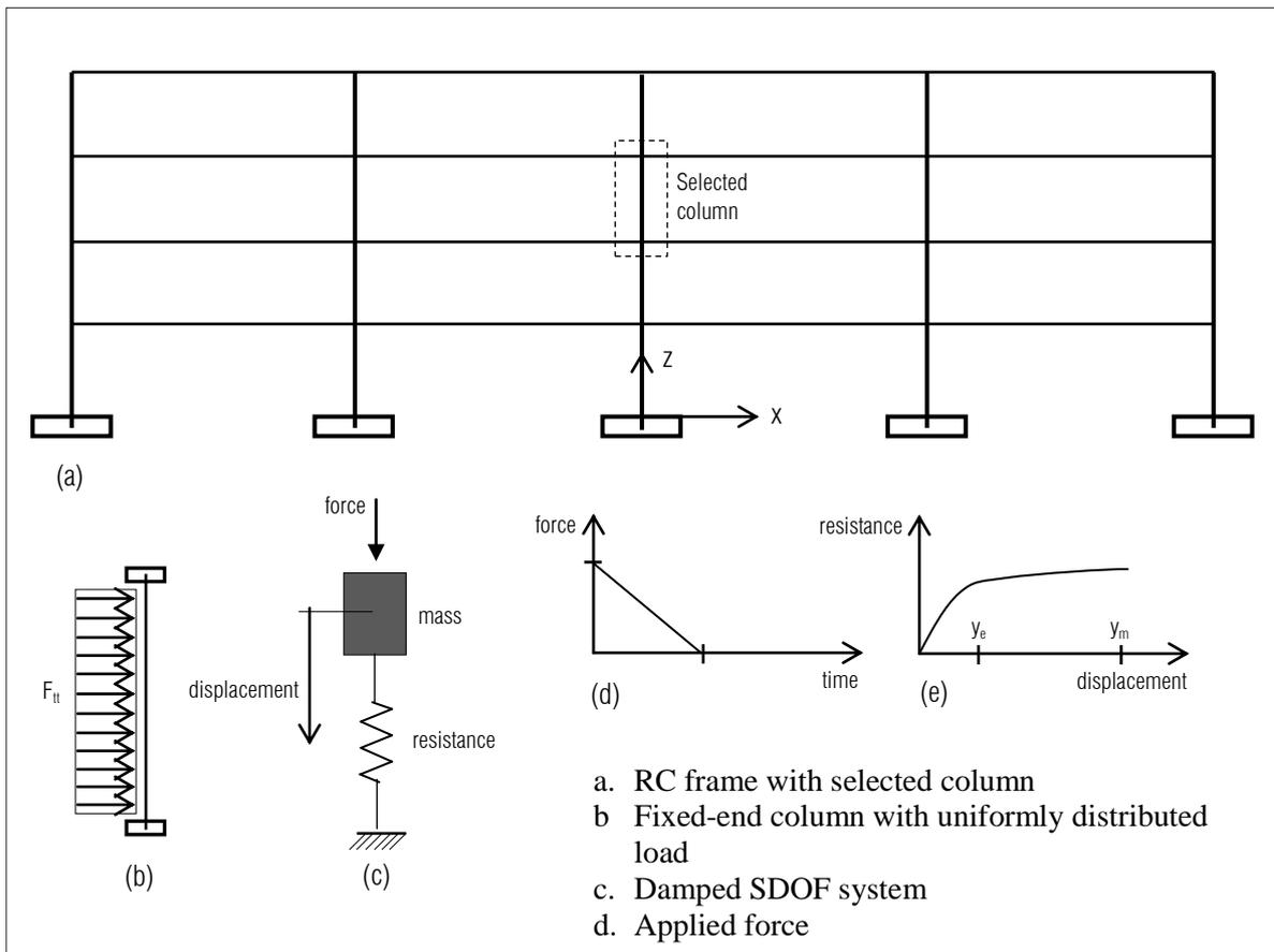
Fig. 6 Equivalent SDOF Model for Dynamic Analysis.
