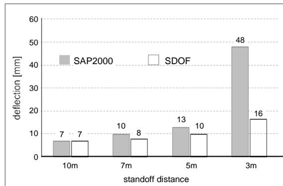
Fig. 8: SAP2000 and A.T.-Blast Comparison of Maximum Displacements
