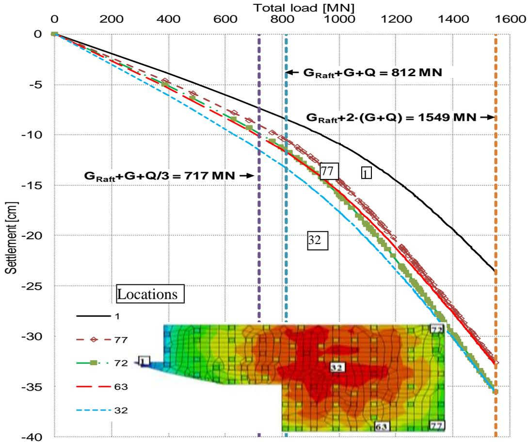
Fig. 8 Load settlement curves at different locations
