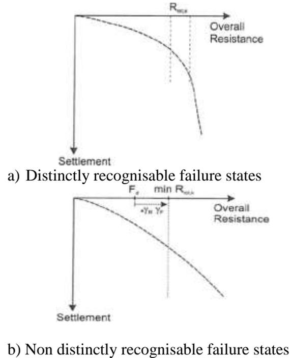
Fig. 2 Non-linear system behaviour of a piled raft and determination of the overall resistance [12]
