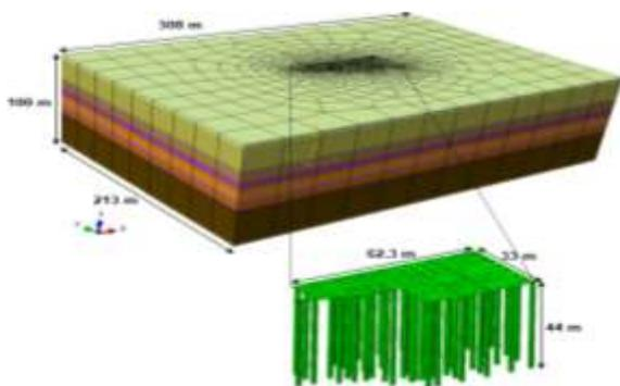
Fig. 7 Geometry of the basic numerical model
