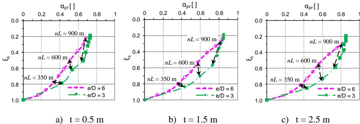
Fig. 7 Variation of the normalized settlement with pile-raft coefficient for different geometric conditions
