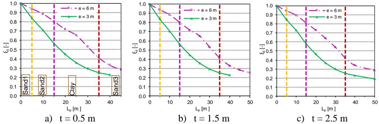
Fig. 5 Variations of the normalized settlement with geometric parameters of the piles and raft.
