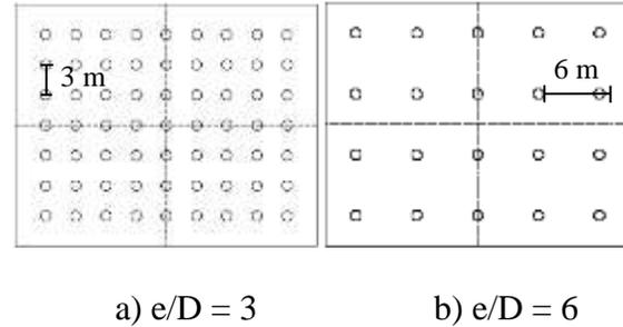
Fig. 4 Pile spacing used for the study
