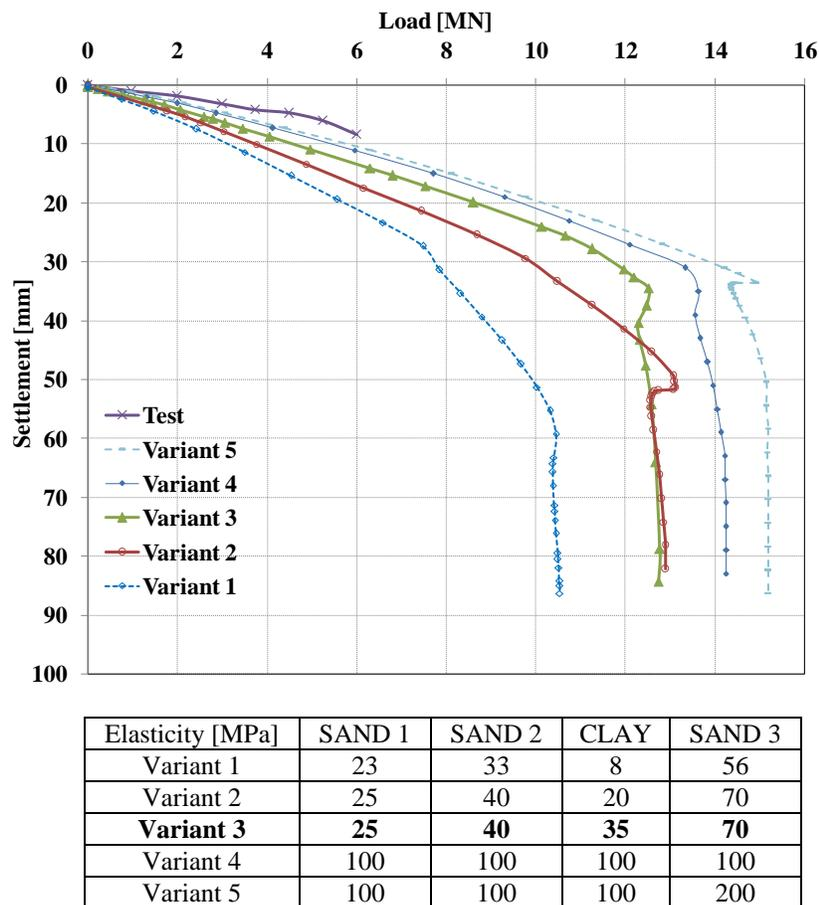
Fig. 3 Calibration of representative static pile-load test using FEM
