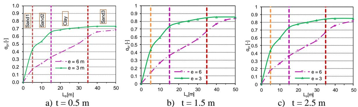
Fig. 6 Variations of the pile raft coefficient with geometric parameters of the piles and raft.
