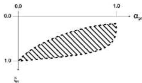
Fig. 1 Relationship between normalized settlement and pile-raft coefficient [4]
