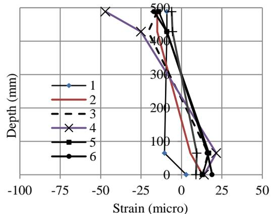
Fig. 7 Stain distribution at 70kN (Position-3)
