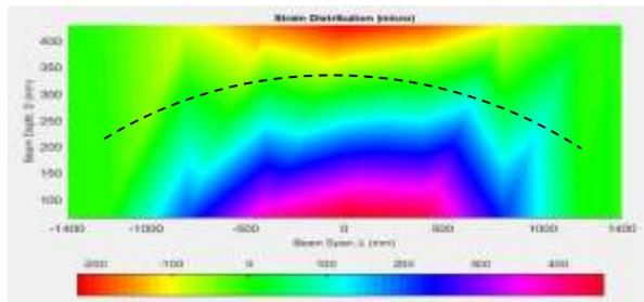
Fig. 14 Stress Distribution (Position-1, Steel at 300kN)
