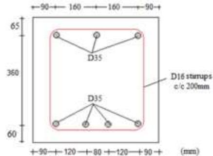
Fig. 2 Cross section of RC beam [9]
