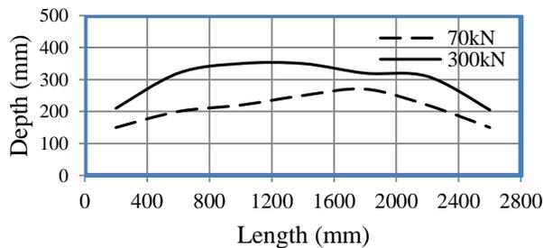
Fig. 9 Variation of NA Profiles (Position-1)
