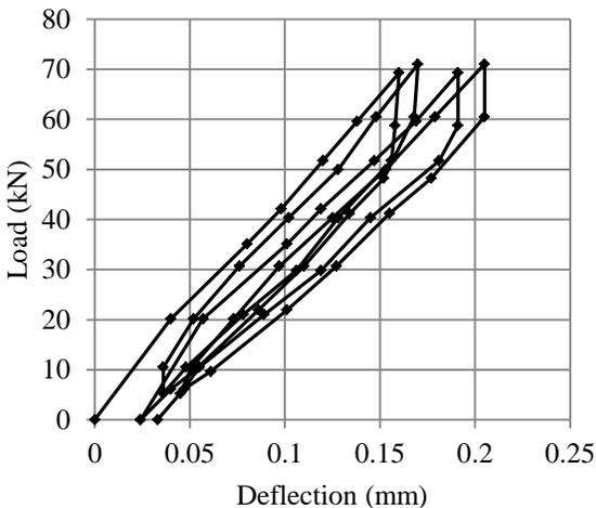
Fig. 4 Load deflection diagram of the test beam due to repeated loading
