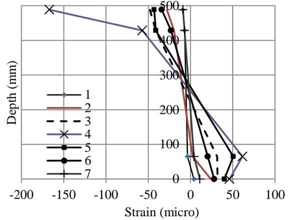
Fig. 5 Stain distribution at 70kN (Position-1)
