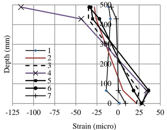
Fig. 6 Stain distribution at 70kN (Position-2)
