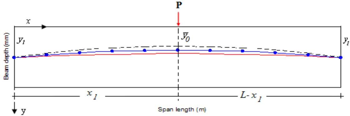
Fig. 1 Concept of variation in neutral axis profile at different loading condition
