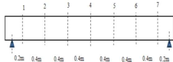
Fig. 3 Locations of strain gauges
