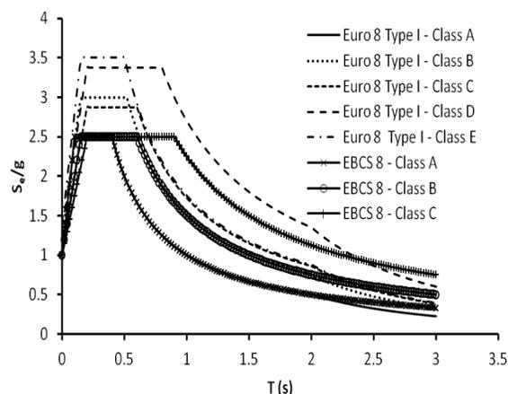
Figure 10 Comparison of EBCS 8 spectra with Type I EC 8: 2004 spectra adapted to 100-year return period
