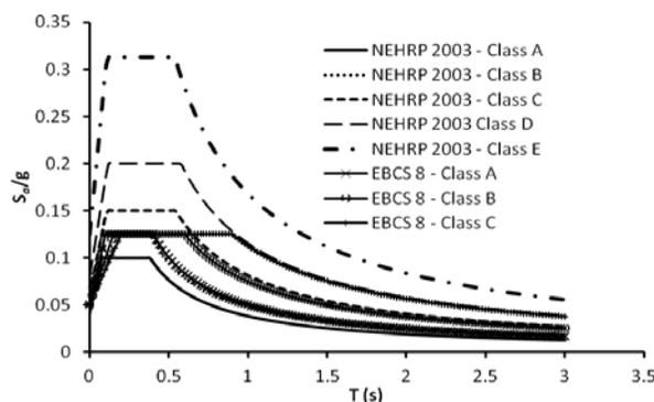
Figure 9 Comparison of EBCS 8 spectra and NEHRP spectra adapted to a return period of 100 years for Zone 2 (including Addis Ababa)
