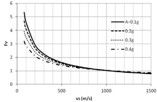
Figure 4 Variation of spectral amplification factors versus  $v_s$  for short and long period ranges and for a range of intensity of rock shaking (Re-plotted after Borcherdt [18])
