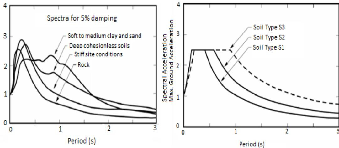
Figure 1. (a) response spectra for different site conditions after Seed et al [12]; (b) The design spectra proposed by ATC-3:1978 Project [16,17]
