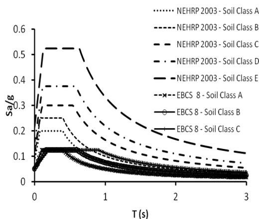
Figure 13 Comparison of EBCS 8 spectra with NEHRP spectra adapted to GSHAP zoning of Ethiopia: Spectra for the second most seismic region (including Addis Ababa)
