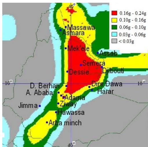
Figure 12 The seismic hazard map of Ethiopia based on the GSHAP data for a return period of 475 years
