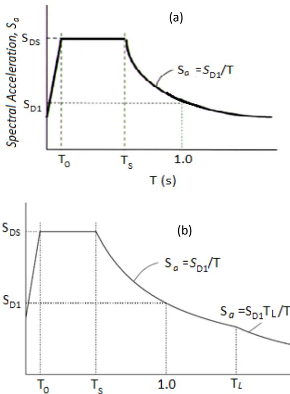
Figure 6 The basic design spectral curves according to (a) NEHRP 1997 [3]; (b) NEHRP 2003[4]
