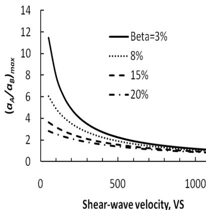
Figure 3 Ground amplification ratio at resonance versus shear-wave velocity for different damping ratios
