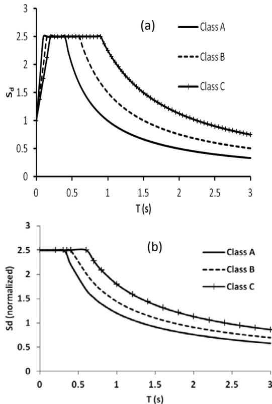
Figure 8 The design spectra of EBCS 8 (1995) (a) for dynamic analysis; (b) for static analysis [1,25]
