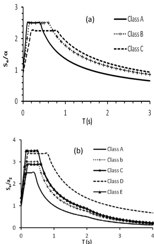
Figure 7 Normalized elastic response spectra: (a) EC 8: 1994 [7]; (b) EC 8: 2004 – Type 1 (for  $M_S \geq 5.5$ ; re-plotted after [8])
