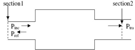
Figure 2 Simple expansion chamber muffler
