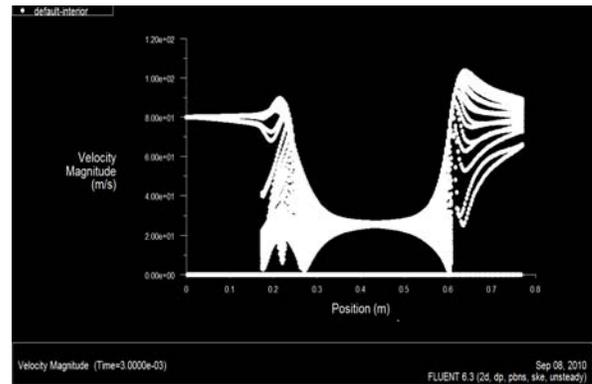
Figure 7 Velocity versus position in muffler
