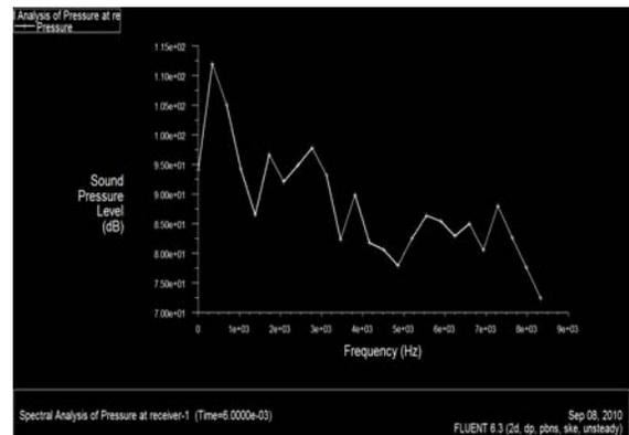
Figure 8 Sound pressure level in dB at the inlet
