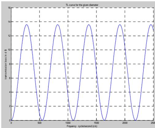
Figure 10 Transmission losses for plane wave equation 1
