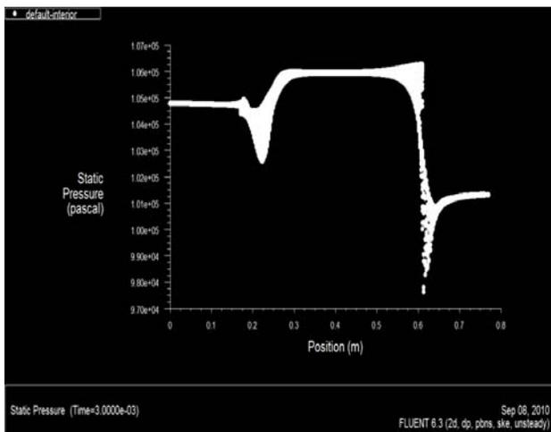
Figure 5 Static pressure versus position in muffler
