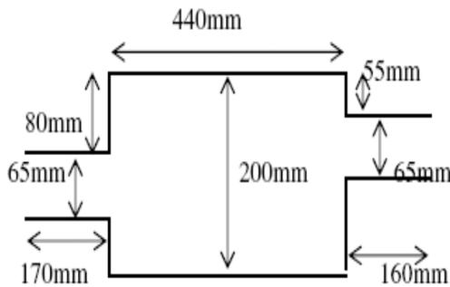
Figure 3 Muffler dimension for simulation
