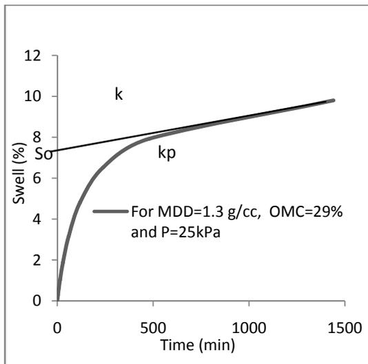
Figure 1 Illustration of Parameter determination for Kality soil
