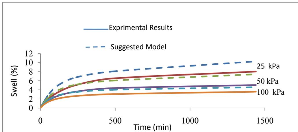
Figure 5 Swell vs. time relationship (MDD=1.3 g/cc and OMC=29 %), soil close to Bole air port.
