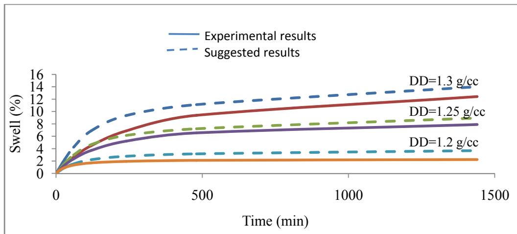
Figure 6 Swell vs. time relationship (OMC=29 % and P=7 kPa), soil close to Bole air port
