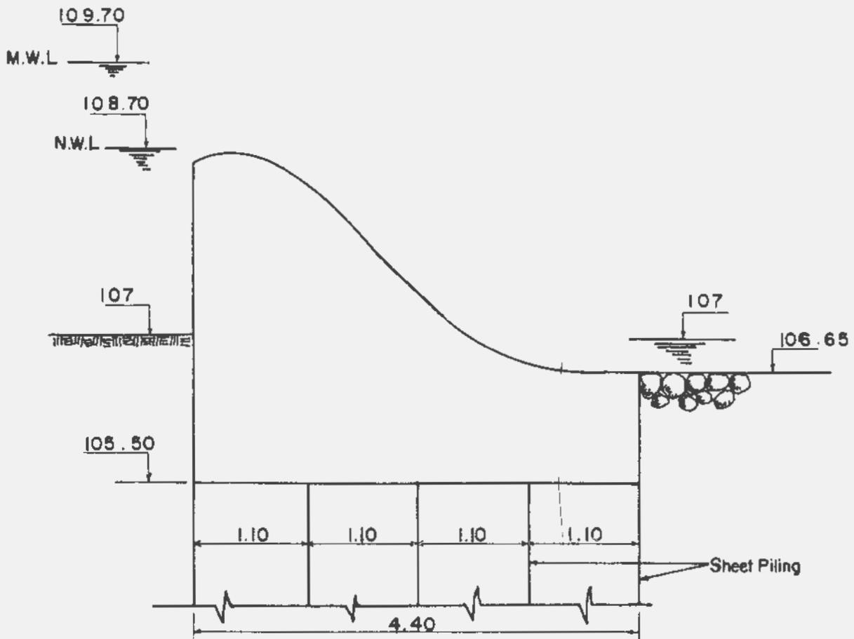
Fig. 1 — Preliminary Design of the Diversion Dam
