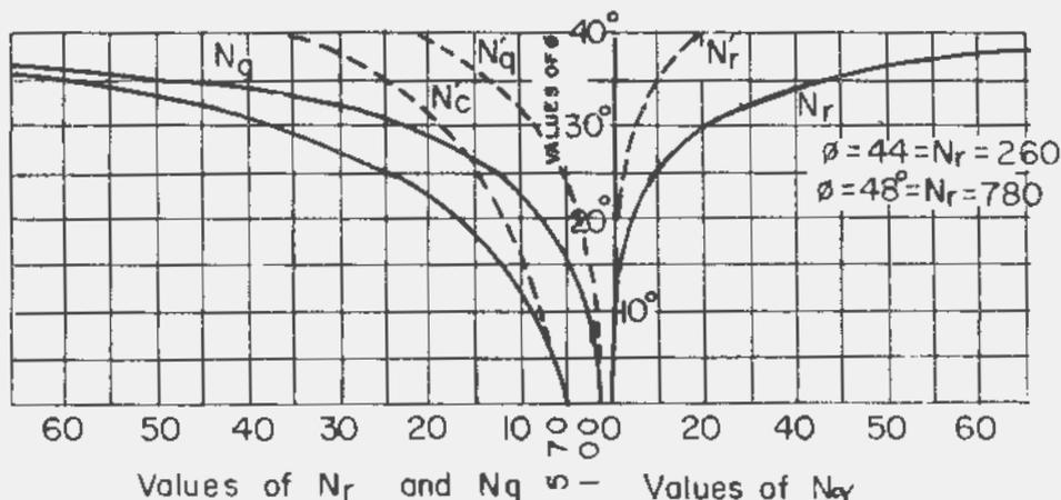
Fig. 5 — Chart showing relation between  $\phi$  and bearing capacity factors
