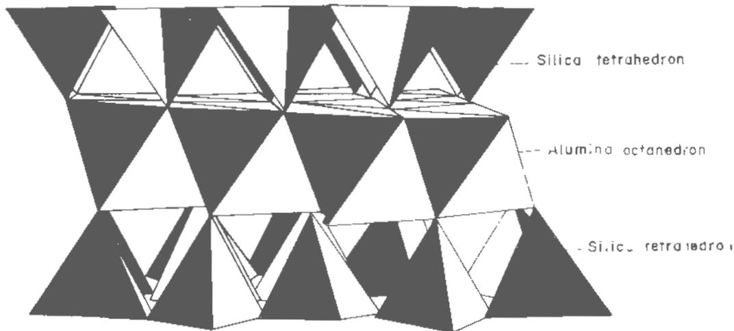
Fig. 1 Model of a Layer of Montmorillonite after Philip Low [4]
