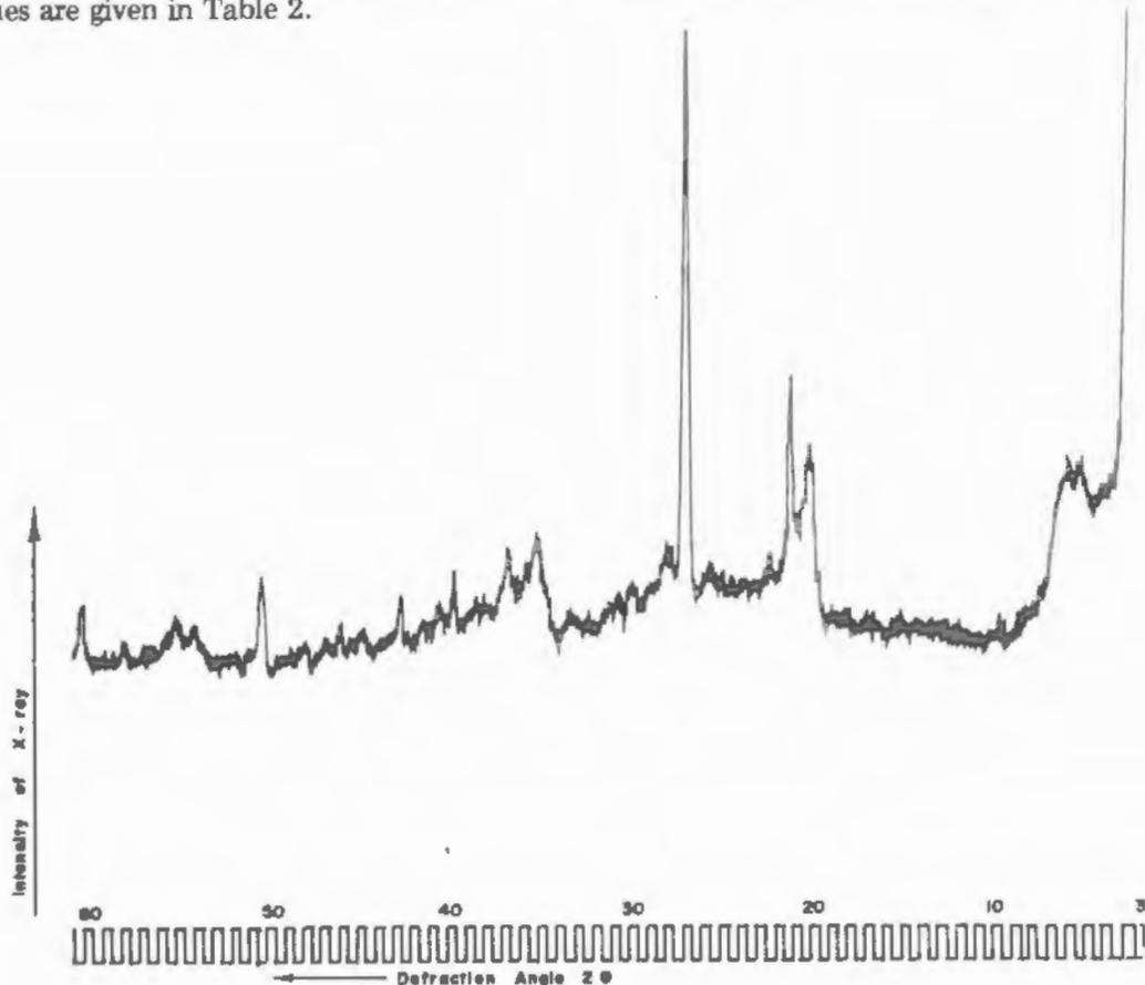
Fig. 3 Typical Result of X-Ray Diffraction Analysis
