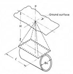
Fig. 6. Concentrated superimposed load
