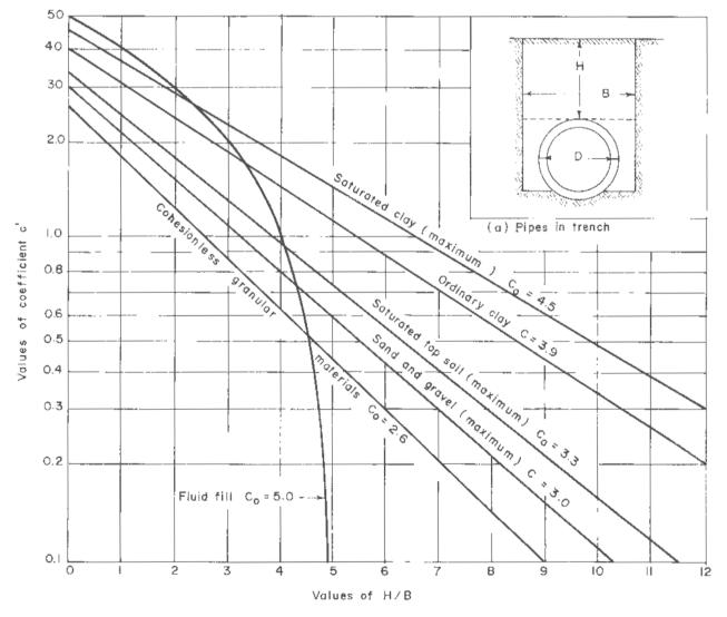
Fig. 4. Vertical External Loads on Circular Conduits
