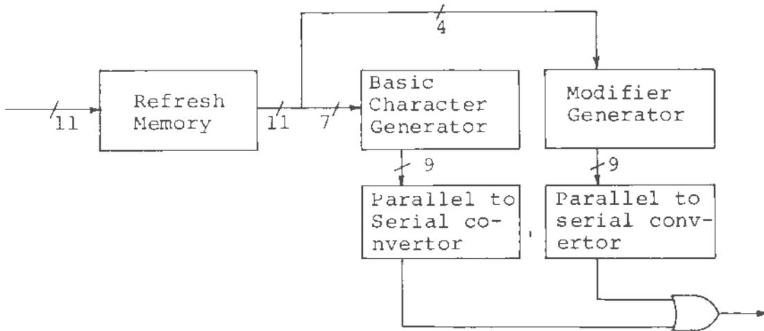
Fig. 2. Character generator using basic EPROM and modifier EPROM
