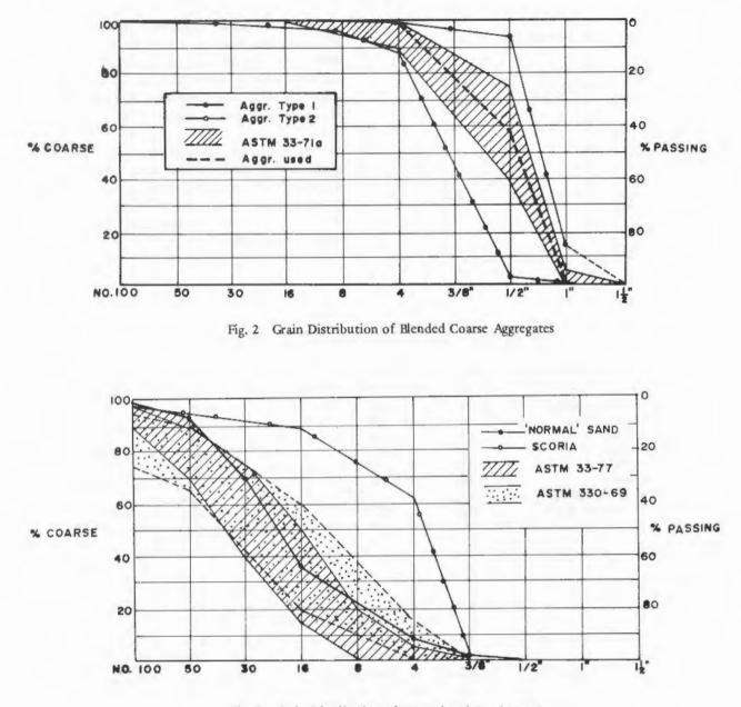
Fig. 3 Grain Distribution of Normal and Scoria Sand
