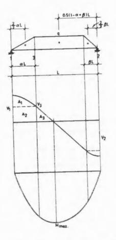
Fig. 1 Shear Force and Bending Moment Diagrams due to Unsymmetrical Trapezoidal Load
