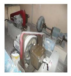
Figure 1 Grinding mill used for grinding and preparing cement (Photo from Mugher Cement Factory Laboratory).
