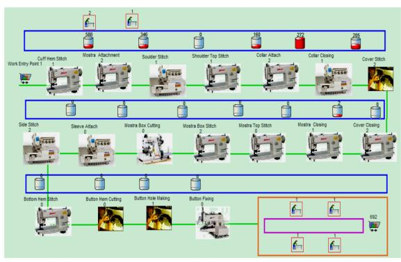
Figure 6 Simulation model of the production line after adding three work centers in the plant
