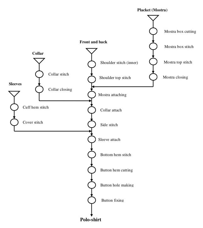
Figure 1 Existing operations of the production system of basic polo-shirt in AAYSC
