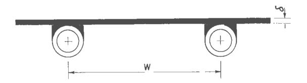
Figure 1 Liquid-cooled Collector Plate and tube Arrangement
