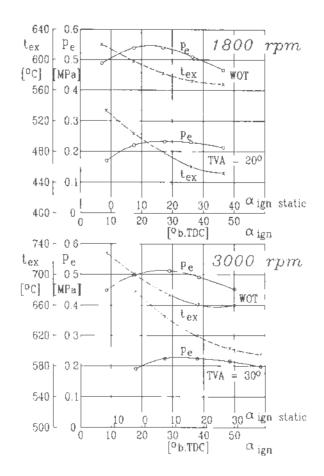
Figure 8 Optimization of Ignition Timing of VW Boxer Engine
