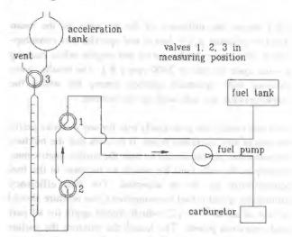
Figure 4 Fuel Consumption Measuring Device
