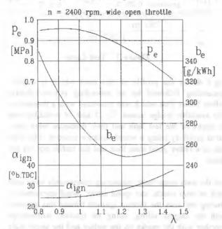
Figure 1 Air Ratio Influence in Engine Parameters
