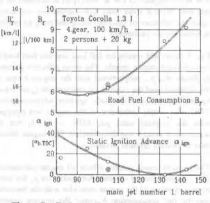
Figure 7 Optimum Road Fuel Consumption
