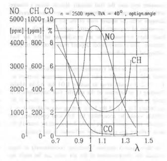
Figure 2 Air Ratio Influence in Exhaust Gas Quality
