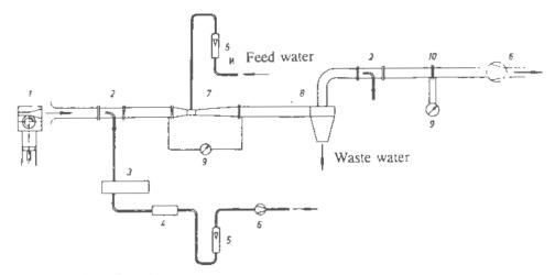
Figure 1 Structure of the Experimental Unit; 1-Dust dosing system, 2-Sampling, 3-Scattered light measuring unit. 4-Filter, 5-Rotameter, 6-Blower, 7-Venture scrubber, 8-Drop separator, 9-Manom. etc. 17 Measuring shade
