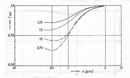
Figure 5 Grade Efficiency with Conical Diffusor Installed at  $u_{LK} = 80$  m/s and  $L = 0.75 \div 1.5.10^3$
