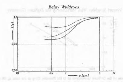
Figure 7: Dependence of the grade efficiency on the diffusor geometry,  $u_{LK} = 70$  m/s,  $L = 1.51 \cdot 10^3$ ; Inv. Parabolic (---), Conical (---) and Parabolic (--)
