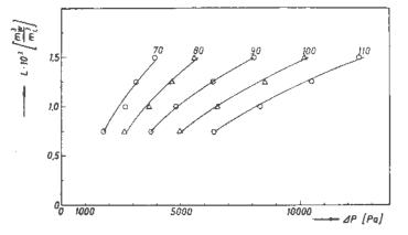
Figure 3 Influence of the Water-Air Ratio and the Throat Velocity on the Pressure Drop for a Conical Difusor with  $u_{lk} = 70 \div 110 \text{ m/s}$
