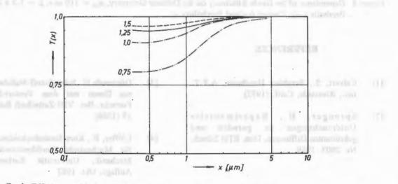
Figure 6 Grade Efficiency with Conical Diffusor Installed at  $u_{LK} = 110$  m/s and  $L = 0.75 \div 1.5 \cdot 10^{-3}$
