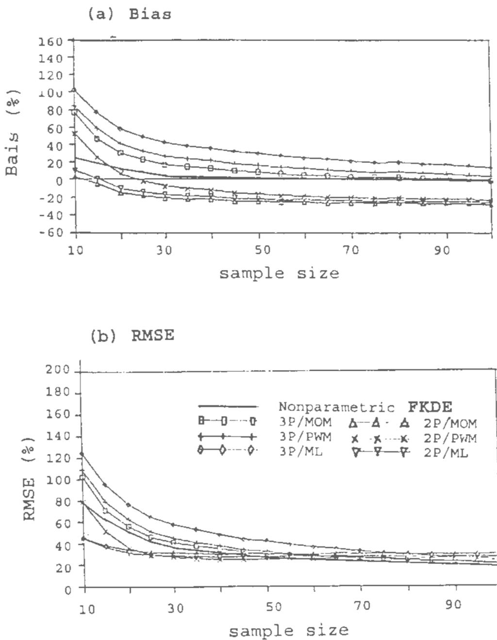
Figure 3 Bias and RMSE of 100 year flow quantile as a function of sample size for population No.1 ( $\theta_1=2.0, \theta_2=1, \theta_3=0.1$  and  $X_{T=100}=0.200$ ), (a) BIAS and (b) RMSE.
