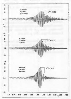
Figure 3 Non-stationary vibration during passage through resonance
