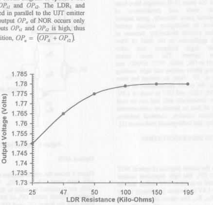
Figure 4. Output Voltage Vs LDR Resistance.
