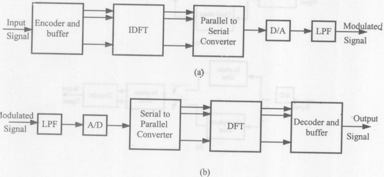
Figure 8 DMT transceiver structure: (a) transmitter (b) receiver
