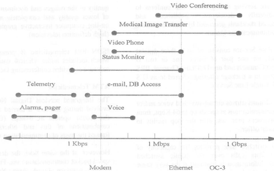
Figure 2 Bandwidth requirement of Telemedicine related application (Bits per second)
