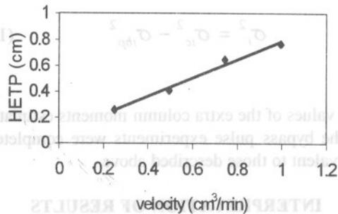
Figure 8 HETP vs fluid velocity for 2.0 g/l betaine concentration
