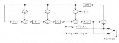
Figure 2 Encoding Circuit for an (n, k) BCH code
