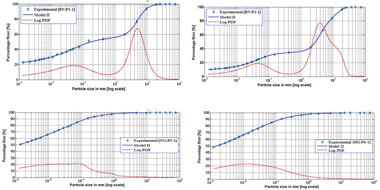
Fig. 12: Typical particle size Log PDF plots with experimental and best-fit curves using Model-II Bimodal fit for representative soil samples
