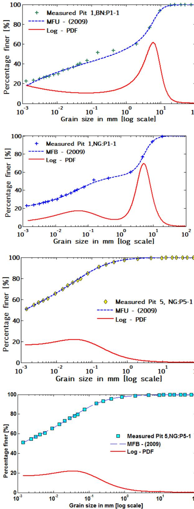
Fig. 4: Typical Particle size Log-PDF plots with experimental and best fit curves using MFU - (2009) and MFB - (2009)
