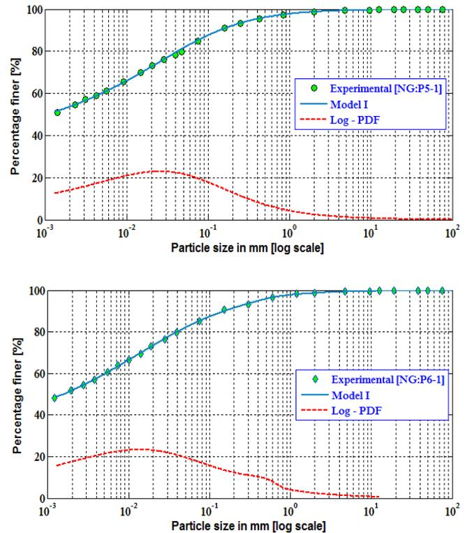
Fig. 8: Typical particle size Log - PDF plots with experimental and best fit curves using Model-I (unimodal model) for various textured soils (Pit 5, NG: P5:1).and (Pit 6, NG: P6:1).
