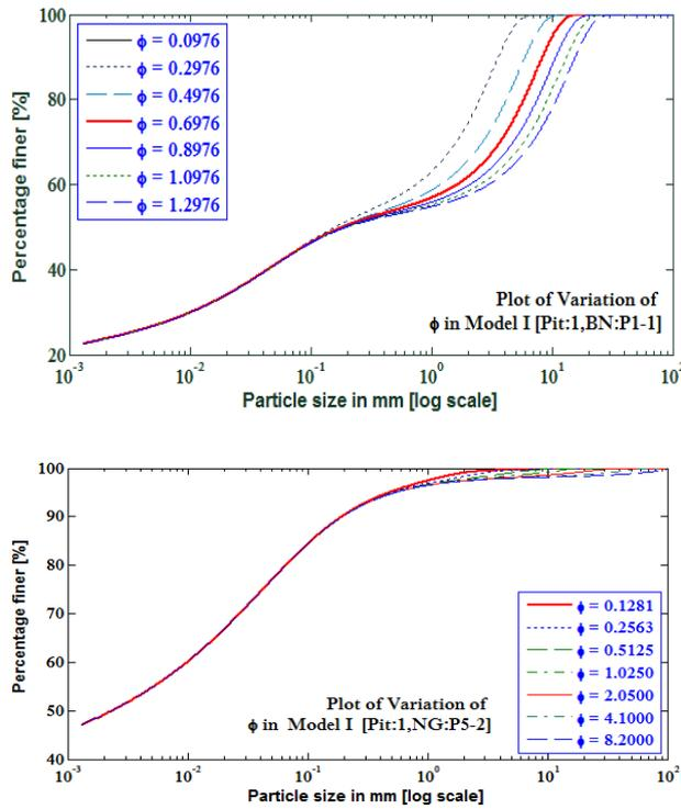
Fig. 11: Effect of varying the  $\phi$  parameter for Model-I, unimodal fit for Pit:1,BN:P1-1:  $\eta = 0.1096$ ,  $\chi = 1.59$  and  $\phi = 0.6976$  and Pit:5, NG:P5-1:  $\eta = 0.098$ ,  $\beta = 0.8749$ ,  $\chi = 2.524E-14$  and  $\phi = 0.1448$ .
