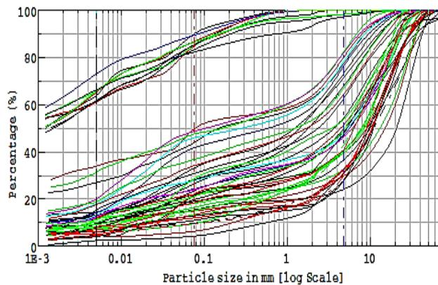
Fig. 1: Particle-size distribution test data on TWR soils used for analysis.
