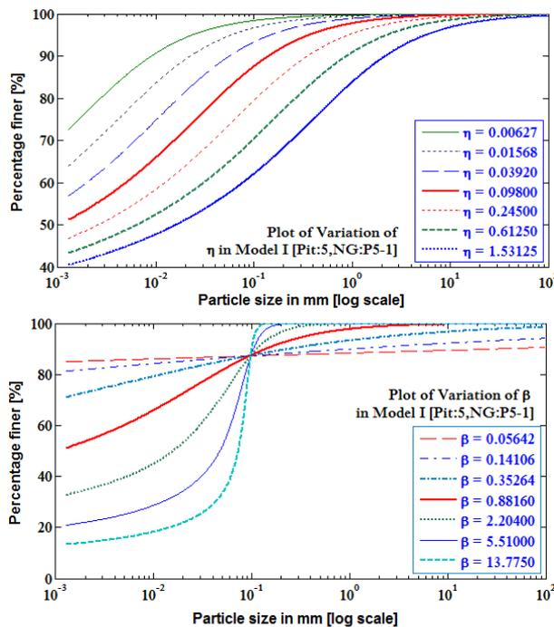
Fig. 9: Effect of varying the  $\eta$  and  $\beta$  parameter for Model-I, unimodal fit for Pit:5, NG: P5-1:  $\eta = 0.0981$ ,  $\beta = 0.8749$ ,  $\alpha = 0.4967$ ,  $\chi = 2.524E-14$  and  $\phi = 0.1448$
