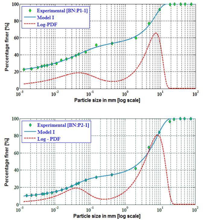
Fig. 7: Typical particle size Log - PDF plots with experimental and best fit curves using Model-I (unimodal model) for various textured soils (Pit: 1, BN: P1-1) and (Pit: 2, BN: P2-1)
