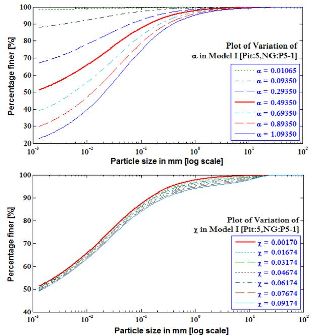
Fig. 10. Effect of varying the  $\alpha$  and  $\chi$  parameter for Model-I, unimodal fit for Pit:5,NG:P5-1:  $\eta = 0.0981$ ,  $\beta = 0.8749$ ,  $\alpha = 0.4967$ ,  $\chi = 2.524E-14$  and  $\phi = 0.1448$ .
