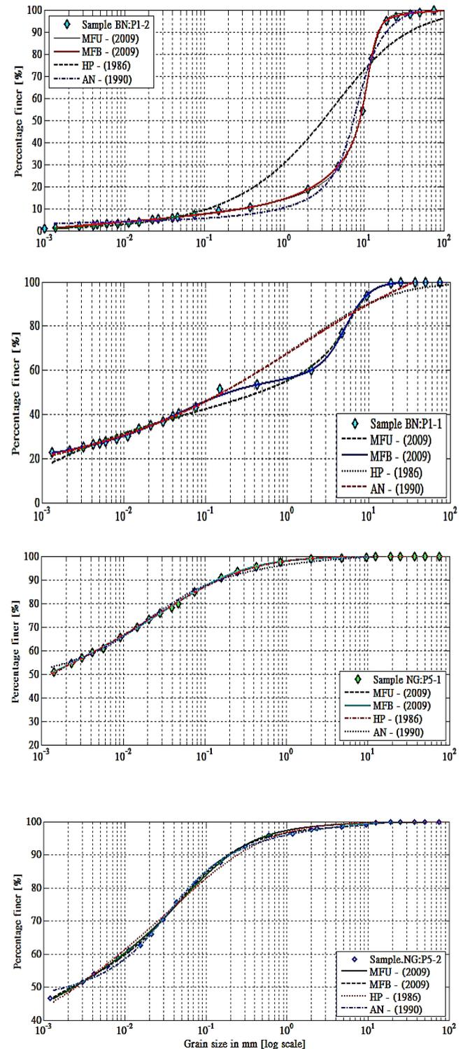
Fig. 2: Typical experimental data fitted using the four PSD models for soils of different gradation
