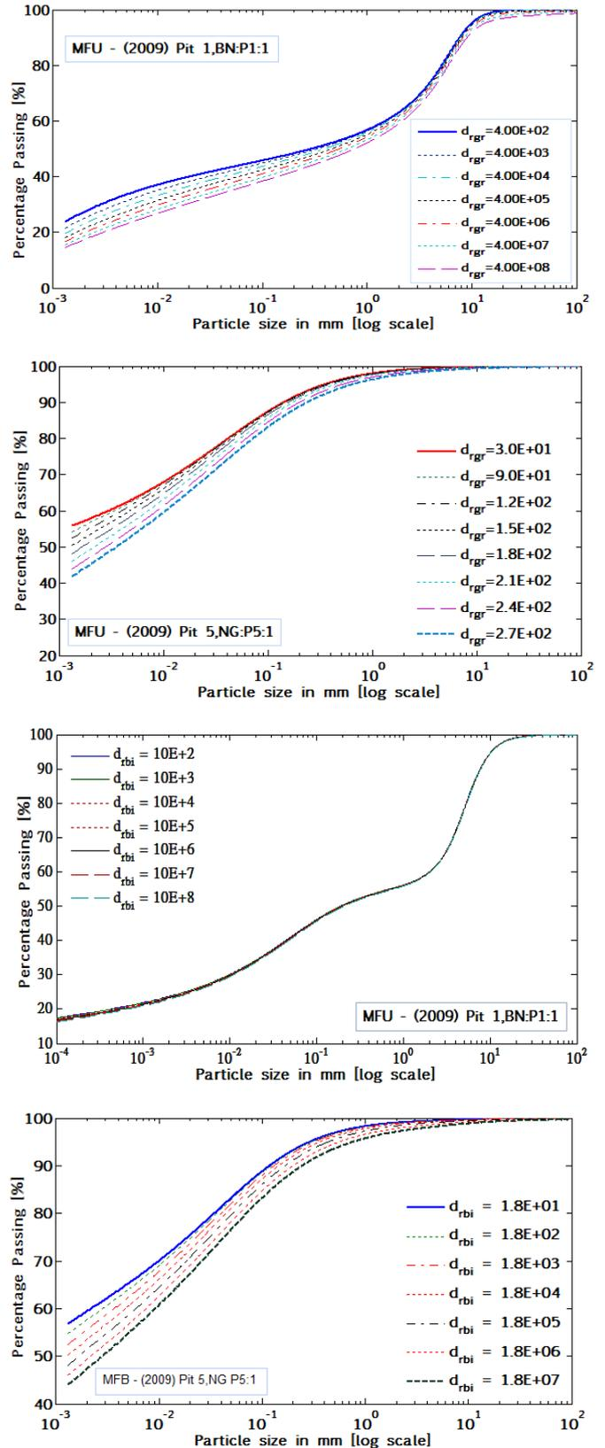
Fig. 5: Effect of varying the  $d_{rgr}$  and  $d_{rbi}$  parameter for MFU - (2009) and MFB - (2009) fit for (Pit: 1, BN: P1-1) and (Pit 5, NG: P5:1).
