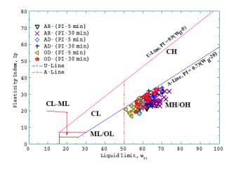
Fig. 18. The locations of the laterite soils studied on the *Casagrande Plasticity Chart*.
