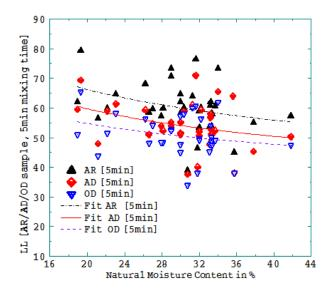
Fig.12. Variations in liquid limits on AR, AD and OD Group B Ethiopian laterite soils tested at *5min* mixing time
