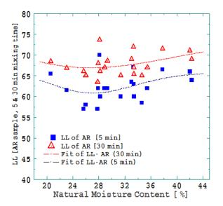
Fig. 7. Variations of liquid limit using AR soil sample tested at 5 and 30min mixing time with natural moisture content for a range of TWR laterite soils tested
