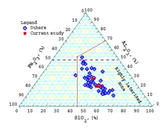
Fig. 5.  $SiO_2 - Al_2O_3 - Fe_2O_3$  triangular diagram indicating the position of the degree of laterization of Ethiopian laterites.
