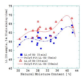
Fig. 9. Variations between liquid limits using OD soil sample tested at 5 and 30min mixing time with natural moisture content for laterite soils tested
