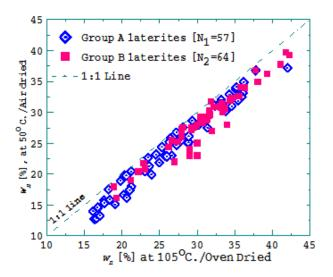
Fig. 6. The relationship between natural moisture content using oven drying of  $50^{\circ}$ C and  $105^{\circ}$ C for a range of *TWR* laterite soils of Ethiopia.
