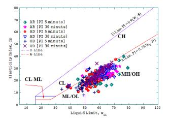
Fig. 19. Locations of Ethiopian laterite soils on the *Casagrande Plasticity Chart* based on several studies (7, 8, 9, 10, 11, 12, 22, 23, 24)
