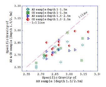
Fig. 14. Line of equality between specific gravity values for ifferent pretest drying treatments
