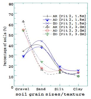
Fig. 15. Variation of the % of the different sizes at different predrying temperature and testing conditions with depth for Group A soils.
