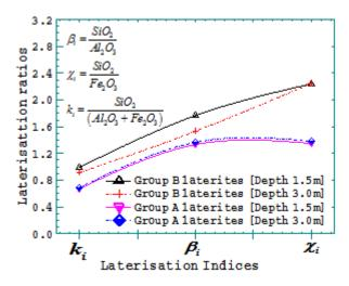
Fig. 4. Average Laterisation indices of Group A and B Ethiopian laterite soils with depth.
